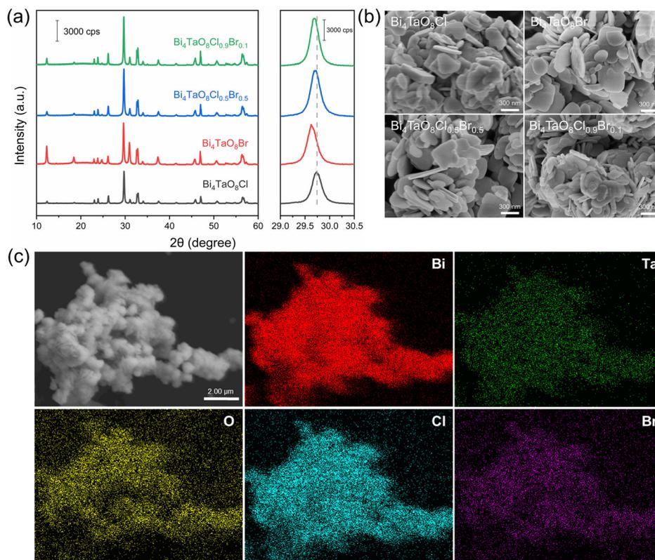
**Fig. 1** (a) XRD patterns and (b) SEM images of  $\text{Bi}_4\text{TaO}_8\text{Cl}$ ,  $\text{Bi}_4\text{TaO}_8\text{Br}$ ,  $\text{Bi}_4\text{TaO}_8\text{Cl}_{0.5}\text{Br}_{0.5}$ , and  $\text{Bi}_4\text{TaO}_8\text{Cl}_{0.9}\text{Br}_{0.1}$ . (c) EDS elemental mapping of  $\text{Bi}_4\text{TaO}_8\text{Cl}_{0.9}\text{Br}_{0.1}$ .
