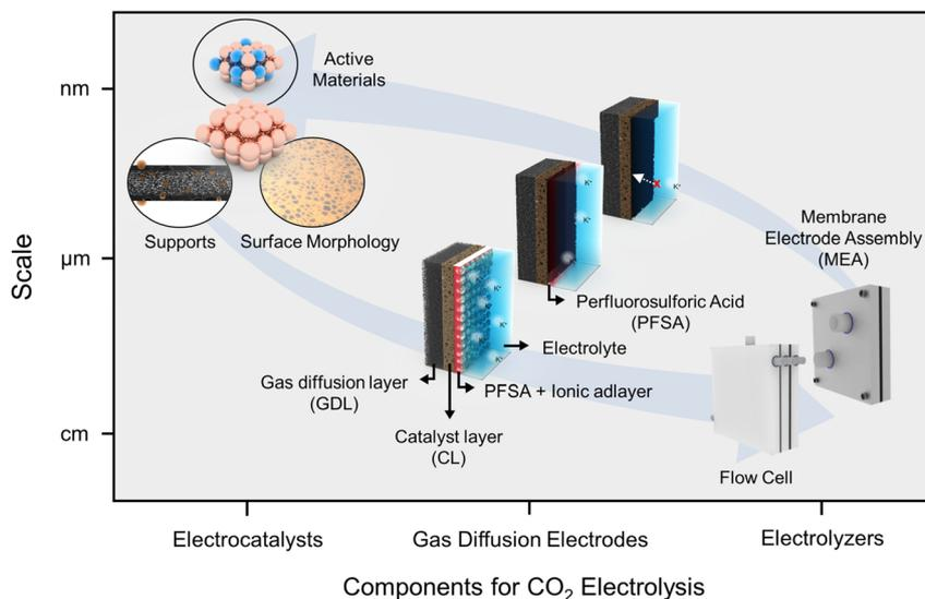
**Fig. 1** Strategic insights into the acidic CO<sub>2</sub>RR in terms of scale and components such as electrocatalysts, gas diffusion electrodes, and electrolyzers.
