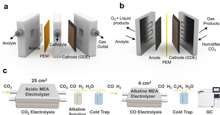
Fig. 7 Application of the acidic CO<sub>2</sub>RR in a tandem electrolyzer system for achieving high SPCE. Schematics of the (a) flow cell and (b) MEA. (c) Zero carbon loss tandem MEA system for MEA to MEA, CO<sub>2</sub> to CO, and CO to C<sub>2</sub>H<sub>4</sub>.<sup>47</sup> Reproduced with permission from ref. 47. Copyright 2023, The Royal Chemical Society.
