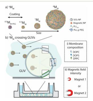
Scheme 1 Magnetic motors that cross lipid membranes. (a) Magnetic motors of different sizes  $({}^xM_M)$  and terminating coatings assembled using the layer-by-layer technique. (b) Giant unilamellar vesicles (GUVs) prepared by varying the membrane composition (i), which affects their fluidity and  $\zeta$ -potential. The ability of  ${}^xM_M$  to cross the lipid membranes of GUVs was evaluated in the presence of different magnetic fields (ii).
