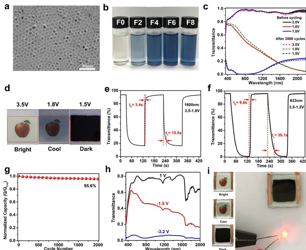
Fig. 5 (a) TEM image and (b) digital photos of  $\text{TiO}_{2-x}$  NCs. (c) Optical transmittance spectra, (d) digital photos, (e and f) switching speed, and (g) cycling stability of  $\text{TiO}_{2-x}$  NC film. (h) Optical transmittance spectra and (i) digital photos of the dual-band EC device. Adapted with permission from ref. 64. Copyright 2020, Wiley-VCH.
