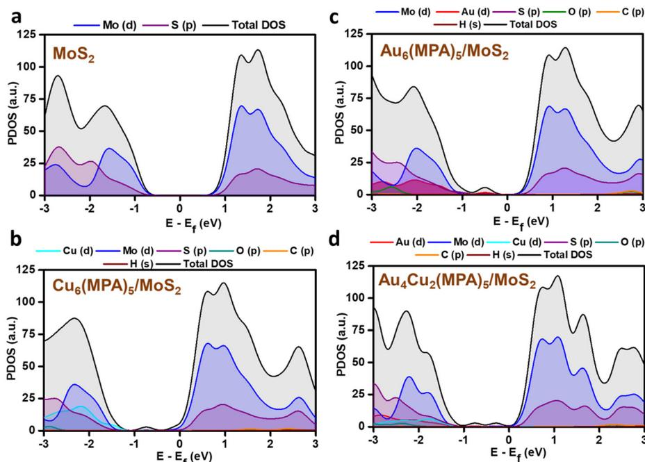
Fig. 7 Partial density of states (PDOS) of (a) pristine MoS<sub>2</sub>, (b) Cu<sub>6</sub>(MPA)<sub>5</sub>/MoS<sub>2</sub>, (c) Au<sub>6</sub>(MPA)<sub>5</sub>/MoS<sub>2</sub>, and (d) Au<sub>4</sub>Cu<sub>2</sub>(MPA)<sub>5</sub>/MoS<sub>2</sub> before H adsorption.
