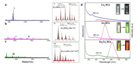
Fig. 1 ESI-mass spectra and corresponding isotopic patterns of (a) Cu<sub>6</sub> NCs, (b)Au<sub>6</sub> NCs, and (c) Au<sub>4</sub>Cu<sub>2</sub>NCs. (d) The corresponding UV-vis absorption and photoluminescence spectra. (Insets show the color of the NCs under visible and UV-light ( $\lambda_{\rm ex} = -365$  nm).).
