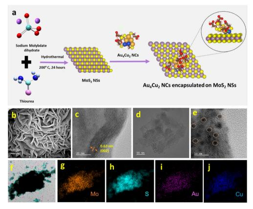
Fig. 2 (a) Schematic illustration of the synthesis of MoS<sub>2</sub> and Au<sub>4</sub>Cu<sub>2</sub>/MoS<sub>2</sub> heterostructures. (b) SEM and (c) HRTEM image of MoS<sub>2</sub> NSs. (d) and (e) TEM and HRTEM images of Au<sub>4</sub>Cu<sub>2</sub>/MoS<sub>2</sub>. (f) STEM image of Au<sub>4</sub>Cu<sub>2</sub>/MoS<sub>2</sub> with the corresponding elemental mappings of (g) Mo, (h) S, (i) Au, and (j) Cu.
