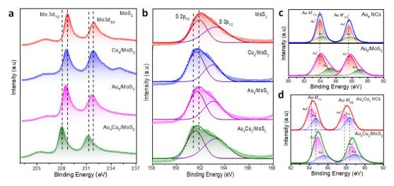
Fig. 3 XPS analysis of MoS<sub>2</sub>,  $Cu_6/MoS_2$ ,  $Au_6/MoS_2$ , and  $Au_4Cu_2NCs/MoS_2$ : (a) Mo 3d, (b) S 2p, (c) XPS spectra of Au 4f in  $Au_6$  NCs and  $Au_6/MoS_2$ , and (d) XPS spectra of Au 4f in Au<sub>4</sub>Cu<sub>2</sub> NCs and Au<sub>4</sub>Cu<sub>2</sub>/MoS<sub>2</sub>.
