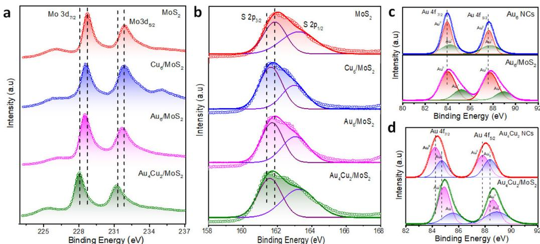
**Fig. 3** XPS analysis of MoS<sub>2</sub>, Cu<sub>6</sub>/MoS<sub>2</sub>, Au<sub>6</sub>/MoS<sub>2</sub>, and Au<sub>4</sub>Cu<sub>2</sub>NCs/MoS<sub>2</sub>: (a) Mo 3d, (b) S 2p, (c) XPS spectra of Au 4f in Au<sub>6</sub> NCs and Au<sub>6</sub>/MoS<sub>2</sub>, and (d) XPS spectra of Au 4f in Au<sub>4</sub>Cu<sub>2</sub> NCs and Au<sub>4</sub>Cu<sub>2</sub>/MoS<sub>2</sub>.
