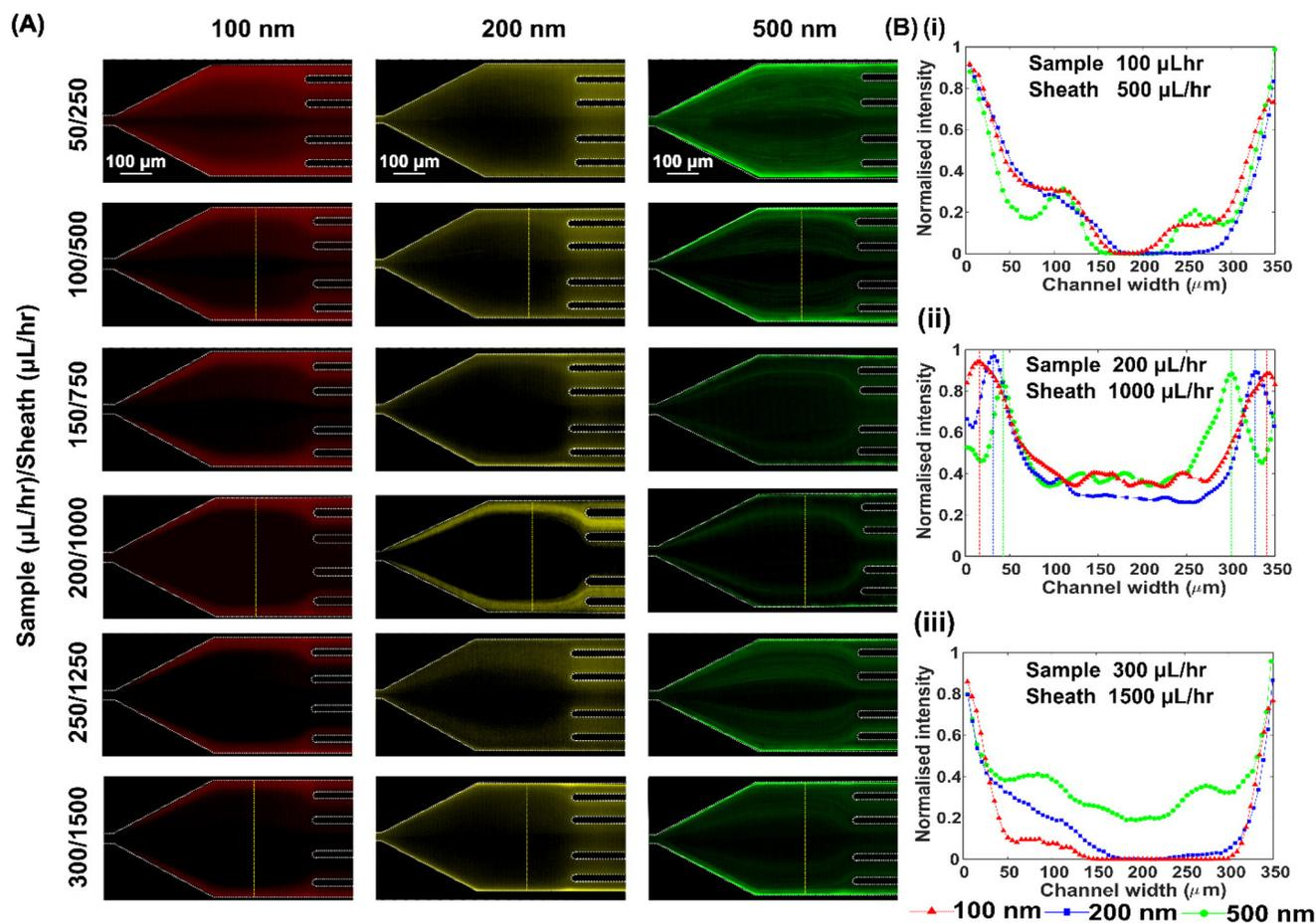
**Fig. 3** (A) Fluorescent trajectories of 100 nm, 200 nm and 500 nm polystyrene particles at the expansion region under total flow rates from 300  $\mu\text{L h}^{-1}$  to 1800  $\mu\text{L h}^{-1}$ . (B) Normalised fluorescence intensity profile across the yellow dotted line at the total flow rate of (i) 600  $\mu\text{L h}^{-1}$ , (ii) 1200  $\mu\text{L h}^{-1}$ , and (iii) 1800  $\mu\text{L h}^{-1}$ . The FRR was constant at 5 : 1 and PEO concentration 1000 ppm.
