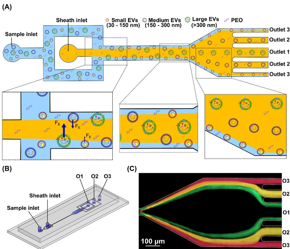
**Fig. 1** (A) Schematic of the size-based separation of EVs in a viscoelastic microfluidic device. (B) A schematic illustration of the microfluidic device. (C) A schematic fluorescence trajectories of 100 nm (pseudo-coloured red), 200 nm (pseudo-coloured yellow) and 500 nm (pseudo-coloured green) polystyrene particles at the expansion region of the channel.
