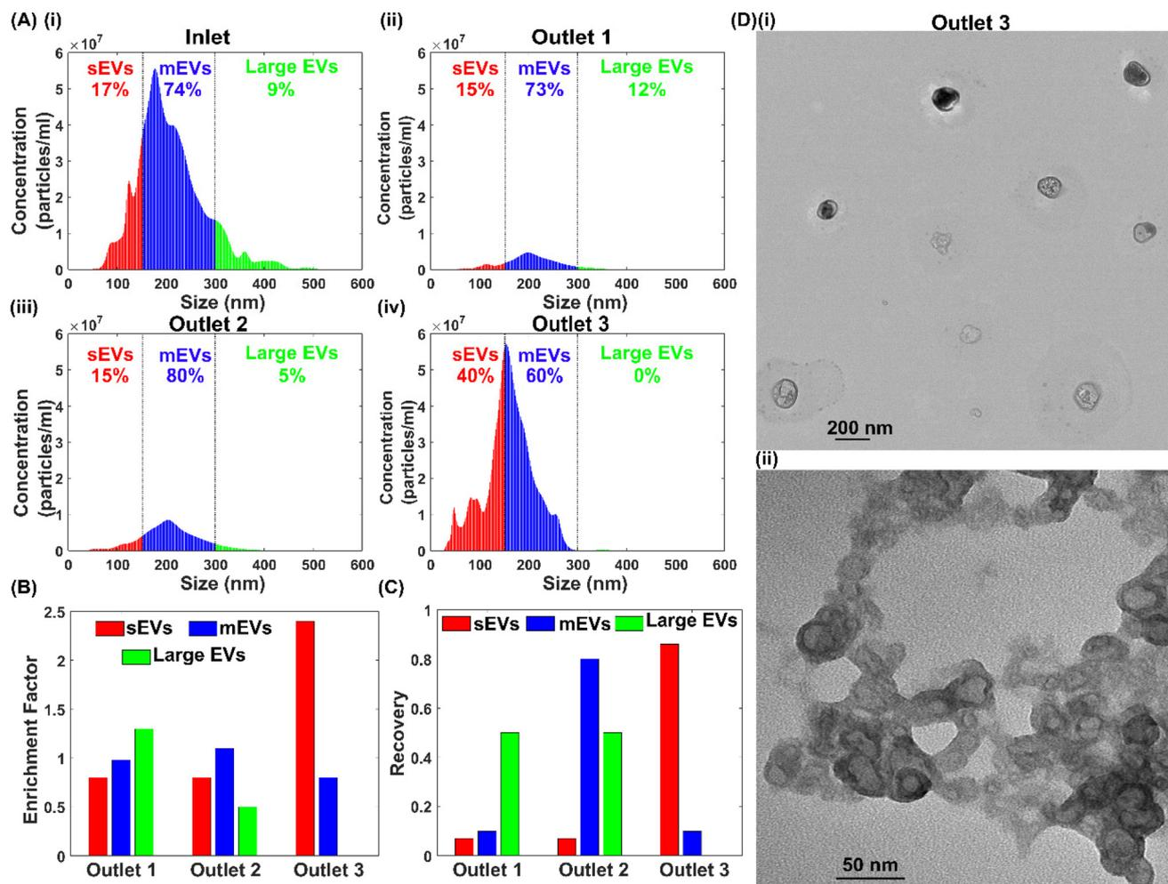
Fig. 6 (A) Size distribution of EVs measured by NTA for inlet and outlets 1–3. (B) The enrichment factor of sEVs, mEVs and large EVs at outlets 1–3. (C) Recovery rates of three EV groups at outlets 1–3. (D) TEM images of EVs from outlet 3 with magnification of (i) 10k and (ii) 80k.
