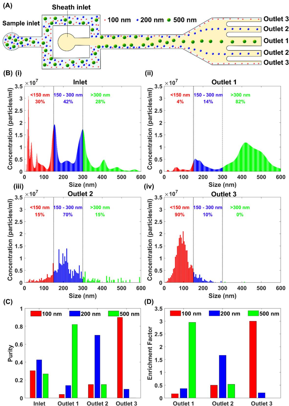
**Fig. 5** (A) Schematics of the size-based separation of 100 nm, 200 nm and 500 nm particles in a viscoelastic microfluidic device. (B) Size distribution of particles measured by NTA for inlet, outlets 1–3. (C) Purity of 100 nm, 200 nm and 500 nm particles at inlet, outlet 1, outlet 2 and outlet 3, respectively. (D) The enrichment factor of 100 nm, 200 nm and 500 nm particles at outlets 1–3.
