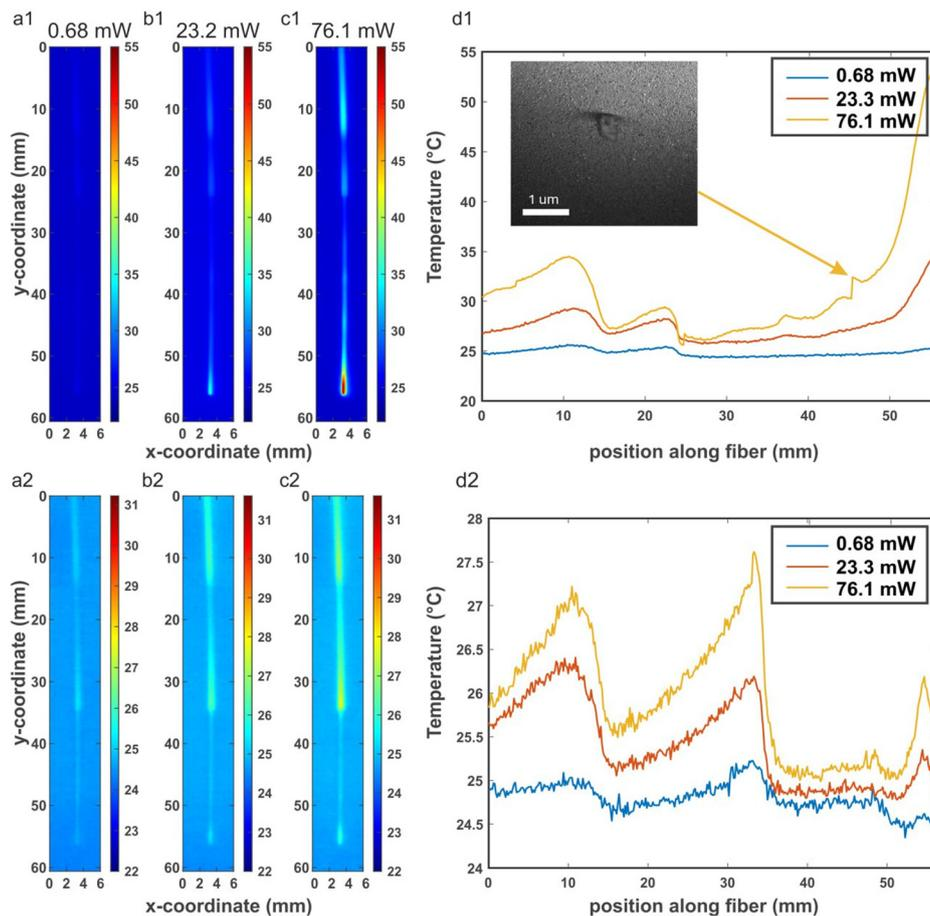
**Fig. 4** Temperature distribution along ordinary and gilded air-filled HCFs. The laser is launched from the bottom facet. The top row (a1, b1 and c1) – gilded fiber. Input laser powers are indicated on the plots. The bottom row – (a2, b2 and c2) the ordinary fiber, the same laser parameters. Panels d1 and d2 are the cuts of the colormaps.
