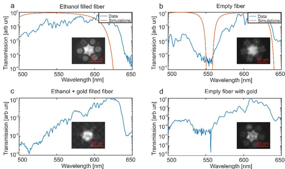
**Fig. 3** Transmission (arbitrary units) spectra of fibers. (a,b) for ethanol and air filled fibers. (c,d) for ethanol and air filled gilded fibers correspondingly. Insets – the CCD image of the optical mode (overall light intensity in the 500–650 nm spectral range).
