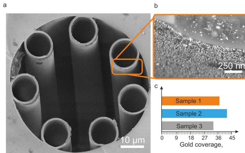
**Fig. 1** (a) SEM image of the HCF with a gold nanoparticle layer deposited on its inner walls. (b) Back scattering electrons (BSE) image of a magnified inner wall surface of a gold-coated fiber; bright spots are Au NPs. (c) Averaged surface coverage of the inner surface of the capillary by Au NPs for 3 different cuts along the fiber.
