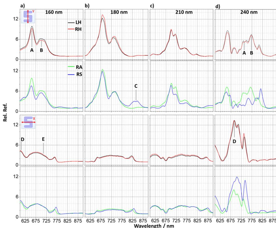
Fig. 2 Experimentally measured *y*- and *x*-polarised relative reflectance for LH (black), RH (red), RA (green) and RS (blue) arrays for silicon structure heights of (a) 160 nm, (b) 180 nm, (c) 210 nm and (d) 240 nm. Peaks of interest are labelled A–E.
