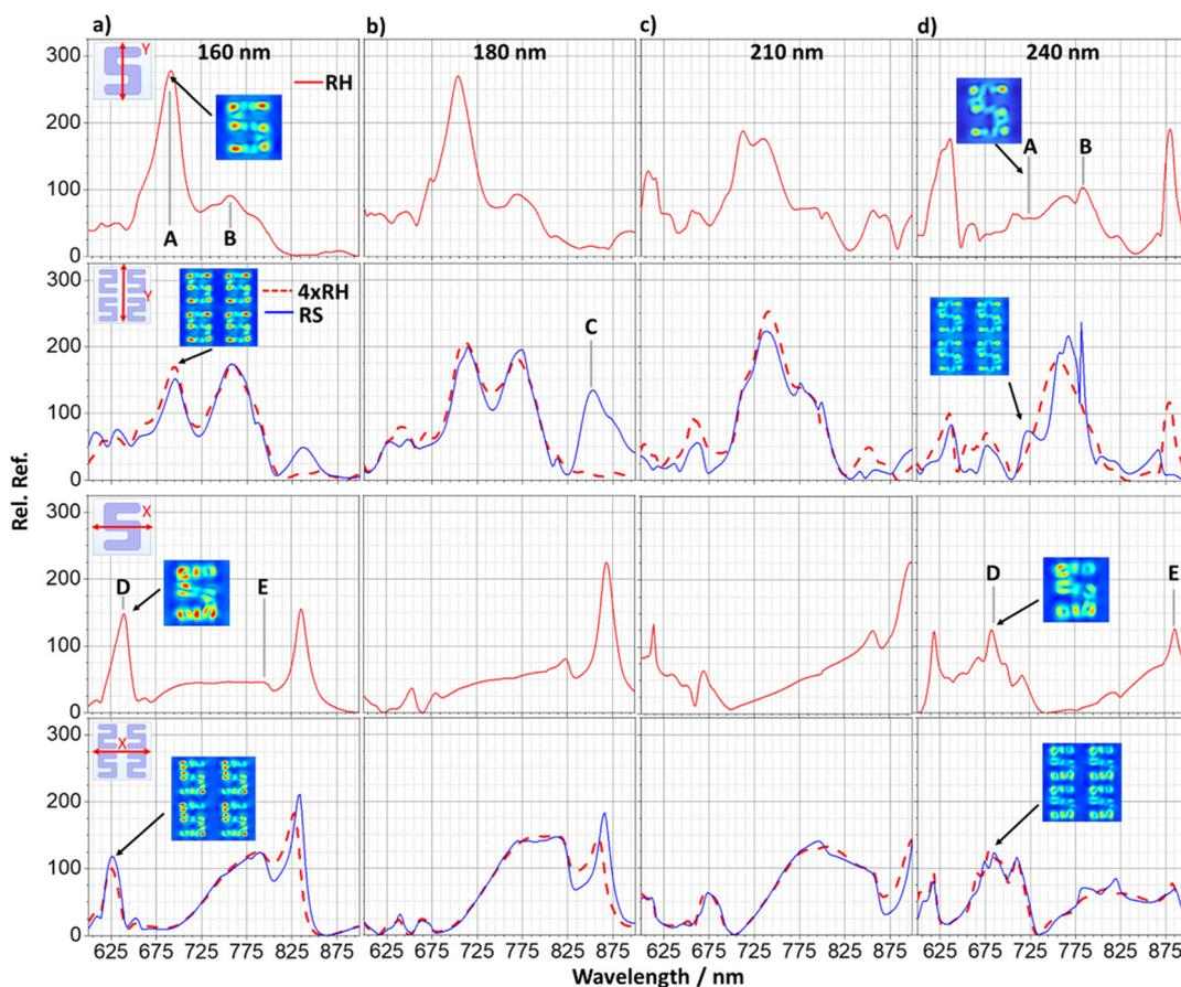
**Fig. 3** Simulated *y*- and *x*-polarised reflectance for each of the 160–240 nm sample heights, (a)–(d). Modelling was performed with a single RH structure (red), four-structured RH models (red dashed) and four-structured RS (blue) arrays. Equivalent peaks with respect to experimental data are labelled A–E. Magnetic field ( $|H|$ ) distribution maps are labelled for equivalent peaks of the two height extremes.
