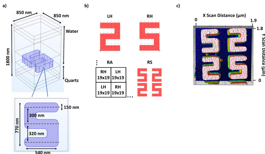
**Fig. 1** (a) The unit cell containing an idealised RH geometry used to model the structures in numerical simulations, with labelled feature sizes. (b) Designs for the repeating units of each array are illustrated. (c) An AFM image of LH and RH structures as part of the RS array.
