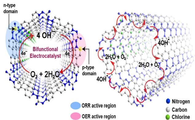
**Fig. 5** Possible mechanism and active site regions for the bifunctional electrocatalysis. Here we represent the simulated structure of vGAC to understand the active sites and probable mechanistic pathways for the ORR and OER in a single framework.
