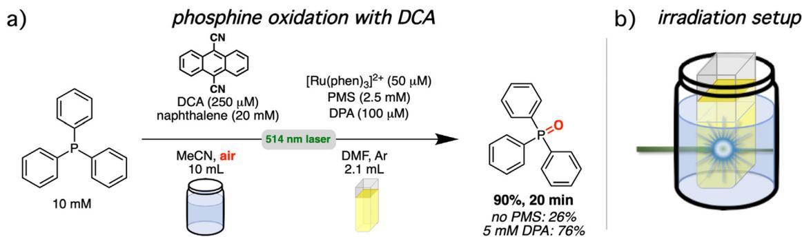
**Fig. 7** Phosphine oxidation *via* green-to-blue sTTA-UC (in argon-saturated solution) and subsequent excitation of 9,10-dicyanoanthracene (DCA) by upconverted light (under aerobic conditions). (a) Reaction conditions under cw laser excitation. Further details and a mechanistic scheme are provided in sections 3.1.2 and 4.6.2 of the ESI.† (b) Schematic representation of the irradiation setup exploiting a two-chamber approach.
