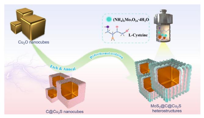
**Scheme 1** Synthetic process of the hollow MoS<sub>2</sub>@C@Cu<sub>2</sub>S heterostructures.
