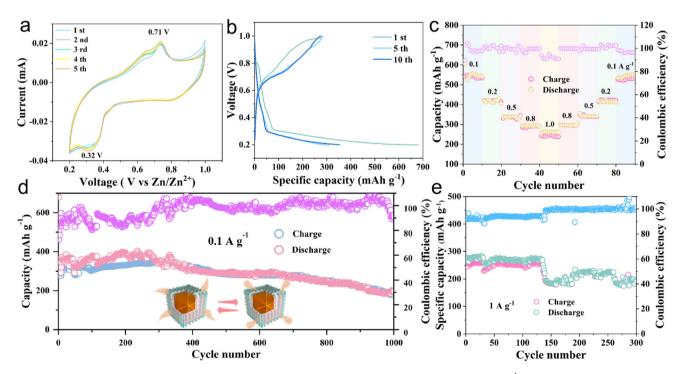
Fig. 2 The electrochemical performance tests of MoS<sub>2</sub>@C@Cu<sub>2</sub>S heterostructures: (a) CV profiles at 0.1 mV s<sup>-1</sup>; (b) charge–discharge curves of the first, fifth and tenth cycles; (c) rate performance; (d) long-term cycling performance; (e) high current density performance.
