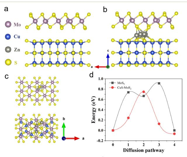
Fig. 4 (a) Optimized structure of MoS<sub>2</sub>@C@Cu<sub>2</sub>S; (b) optimized structure of Zn<sup>2+</sup> insertion in MoS<sub>2</sub>@C@Cu<sub>2</sub>S; (c) top view of the optimized structure ture of Zn<sup>2+</sup> insertion in pure MoS<sub>2</sub> and MoS<sub>2</sub>@C@Cu<sub>2</sub>S; (d) energy barriers of diffusion behavior of Zn<sup>2+</sup> in pure MoS<sub>2</sub> and MoS<sub>2</sub>@C@Cu<sub>2</sub>S.
