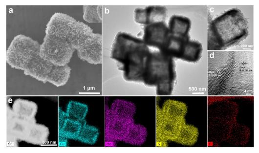
Fig. 1 Characterization of MoS<sub>2</sub>@C@Cu<sub>2</sub>S heterostructures: (a) SEM image; (b-d) TEM images; (e) elemental mapping images.
