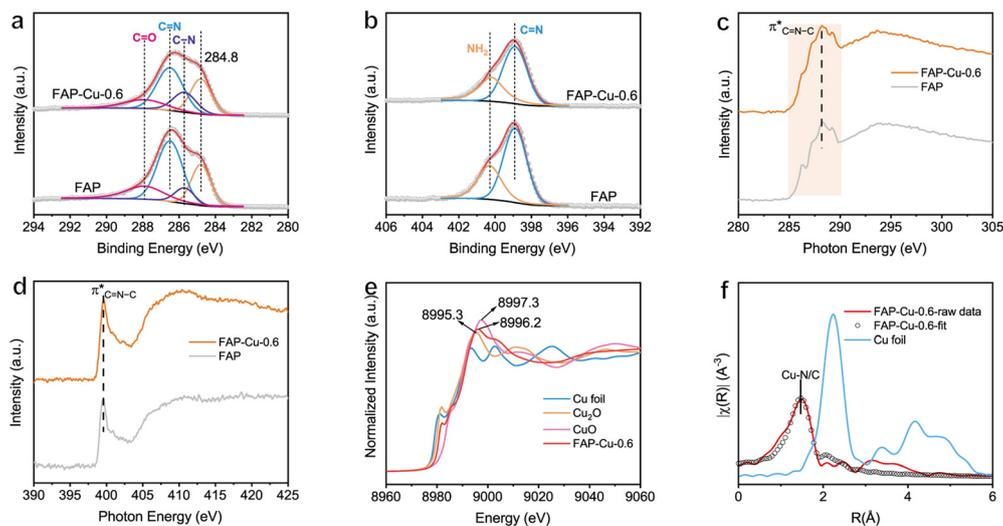
**Fig. 2** (a) C 1s and (b) N 1s XPS spectra of FAP and FAP-Cu-0.6. (c) C K-edge and (d) N K-edge XAS spectra of FAP and FAP-Cu-0.6. (e) Cu K-edge XANES spectra and (f) the  $k^2$ -weighted FT-EXAFS spectra of FAP-Cu-0.6.
