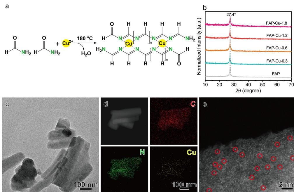
**Fig. 1** (a) A schematic illustration of the synthesis of a single-atom Cu catalyst supported on a formamide polymer. (b) XRD patterns of the FAP and FAP-Cu- $x$  catalysts. (c–e) TEM image (c); EDS elemental mapping images of C, N and Cu elements (d); and aberration-corrected HAADF-STEM image (e) of the FAP-Cu-0.6 sample.
