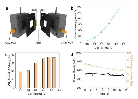
Fig. 4 (a) A schematic illustration of the MEA electrolyzer. (b) Current densities and (c) related CH<sub>4</sub> FEs in the MEA electrolyzer under different cell potentials over the FAP-Cu-0.6 catalyst. (d) The chronoamperometric stability test for the MEA electrolyzer.
