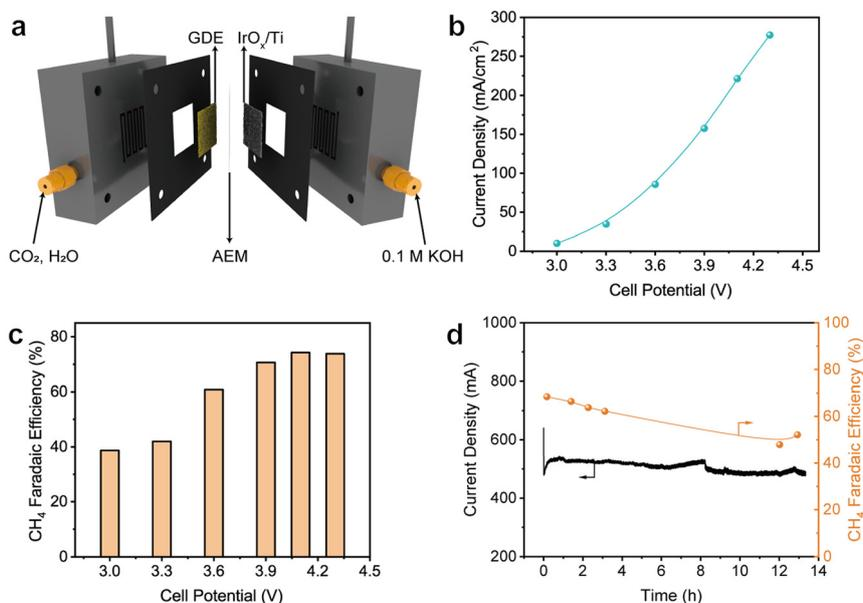
**Fig. 4** (a) A schematic illustration of the MEA electrolyzer. (b) Current densities and (c) related  $\text{CH}_4$  FEs in the MEA electrolyzer under different cell potentials over the FAP-Cu-0.6 catalyst. (d) The chronoamperometric stability test for the MEA electrolyzer.
