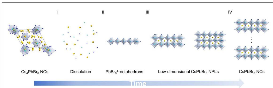
Fig. 6 Schematic illustration of the proposed transformation mechanism.
