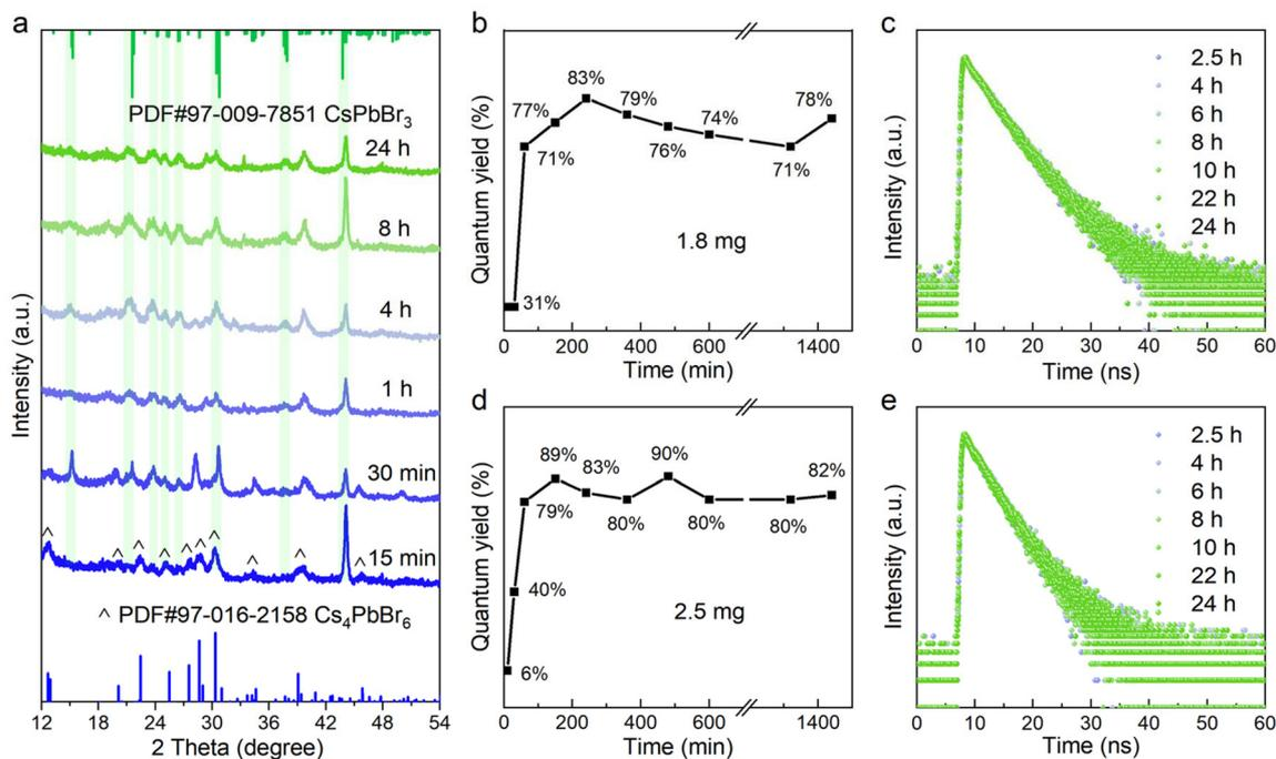
Fig. 3 (a) XRD patterns of the luminescent products synthesized with 1.8 mg NOBF<sub>4</sub> at different reaction times. (b and d) Quantum yield and (c and e) PL decay spectra of the luminescent products synthesized with 1.8 mg and 2.5 mg NOBF<sub>4</sub> at different reaction times.
