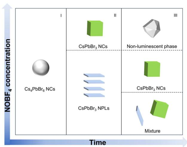
Fig. 2 Schematic presentation of the nanostructures in the reaction medium with the reaction time and NOBF<sub>4</sub> concentration.
