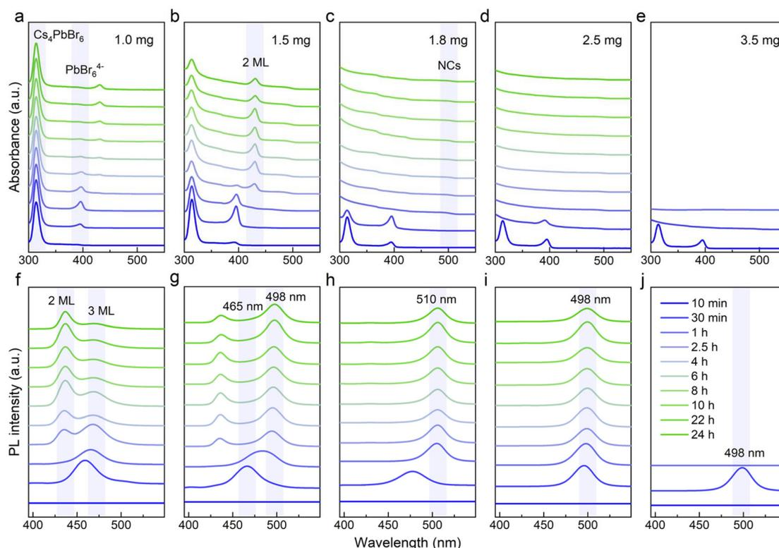
**Fig. 1** (a–e) Absorption and (f–j) PL spectra of luminescent products obtained with different amounts of NOBF<sub>4</sub> (1.0 mg, 1.5 mg, 1.8 mg, 2.5 mg and 3.5 mg) at different reaction times.
