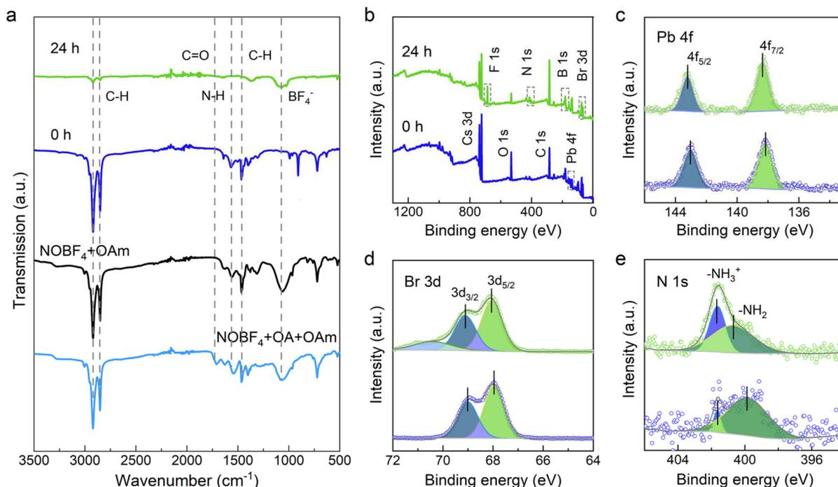
**Fig. 5** (a) FTIR and (b) full XPS spectra of pristine  $\text{Cs}_4\text{PbBr}_6$  NCs (0 h) and the newly formed  $\text{CsPbBr}_3$  NCs after 24 h with 1.8 mg  $\text{NOBF}_4$ . High-resolution XPS spectra of (c) Pb 4f, (d) Br 3d and (e) N 1s.
