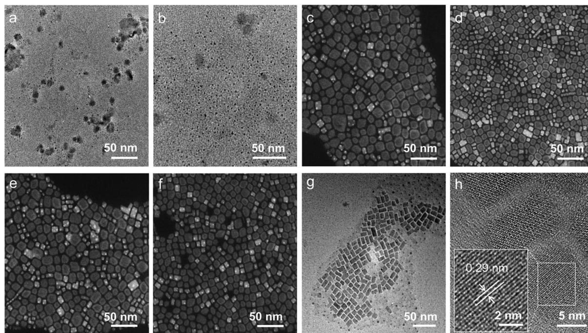
Fig. 4 (a–f) TEM images of the luminescent products obtained with 1.8 mg  $\text{NOBF}_4$  at 15 min, 30 min, 1 h, 4 h, 8 h and 24 h. (g) TEM and (h) HRTEM images of the purified luminescent products obtained with 1.8 mg  $\text{NOBF}_4$ .
