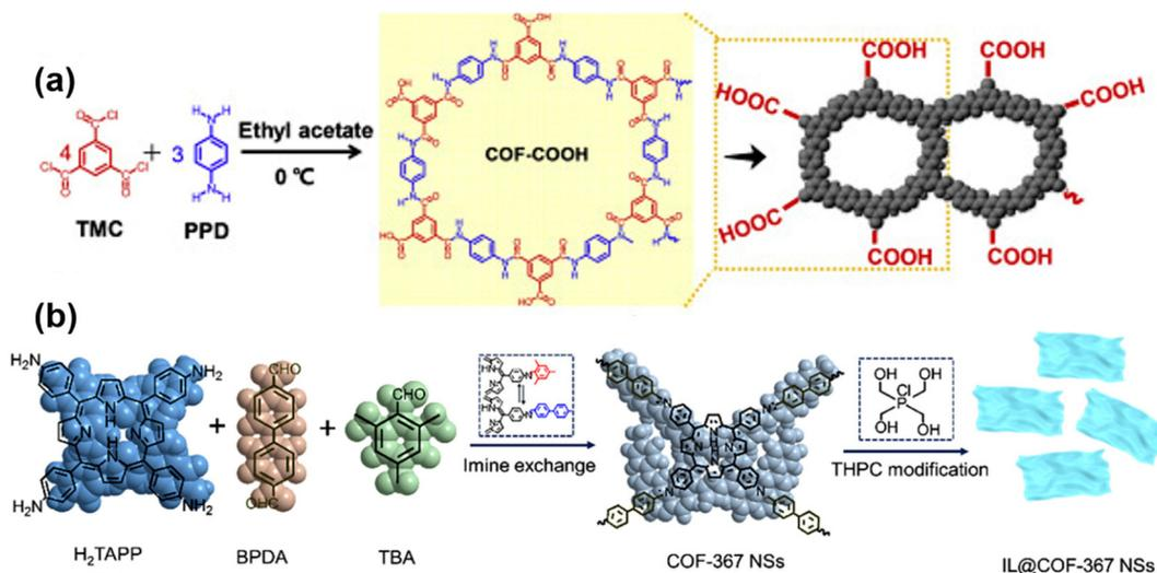
**Fig. 8** (a) Schematic illustration of the preparation of COF-COOH membrane. Reproduced with permission from ref. 85. Copyright 2020, published by Elsevier B.V. (b) Diagrammatic drawing of the synthetic procedure for the COF-367 and IL@COF-367 NSs. Reproduced with permission from ref. 86. Copyright 2022, Elsevier B.V. All rights reserved.
