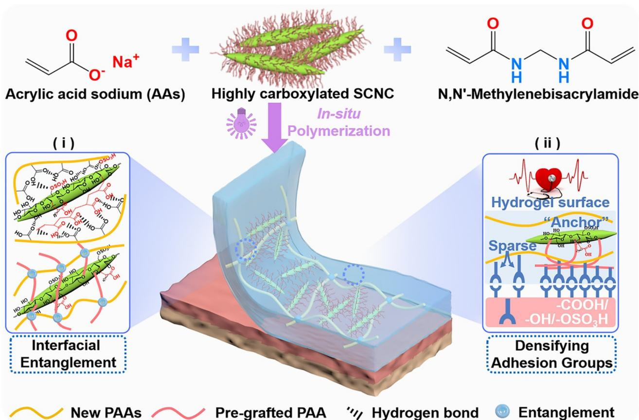
Fig. 1 A schematic illustration of the fabrication and network structure of the tough, highly adhesive/conductive nanocomposite hydrogel patch (PACP<sub>x</sub>H; X is the content of SCNCPA).
