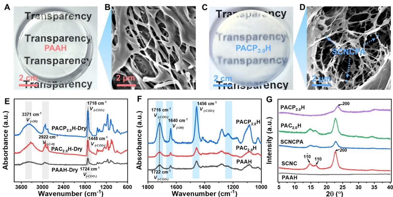
**Fig. 2** (A and C) The optical images of PAAH and PACPH. (B and D) The SEM images of PAAH and PACPH after freeze-drying. (E) The FTIR spectra of PAAH, PACH and PACPH after freeze-drying. (F) The Raman spectra of the three hydrogels in the aqueous state (considering the effect of water on hydrogen bonding). (G) The XRD spectra of SCNC and SCNCPA powders and the three hydrogels after freeze-drying.
