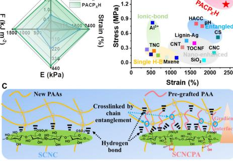
Fig. 4 (A) The radar plot of the comprehensive mechanical properties of PACPH. (B) Comparison of the maximum tensile strength and strain at break of PACPH with the currently used PAA-based hydrogels. (C) Strengthening and toughening mechanism of SCNCPA with abundant carboxylate groups on the surface and the gradient structure (pre-grafted molecular chains) in a single hydrogel network.
