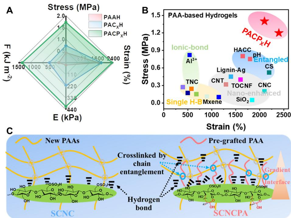
**Fig. 4** (A) The radar plot of the comprehensive mechanical properties of PACPH. (B) Comparison of the maximum tensile strength and strain at break of PACPH with the currently used PAA-based hydrogels. (C) Strengthening and toughening mechanism of SCNCPA with abundant carboxylate groups on the surface and the gradient structure (pre-grafted molecular chains) in a single hydrogel network.
