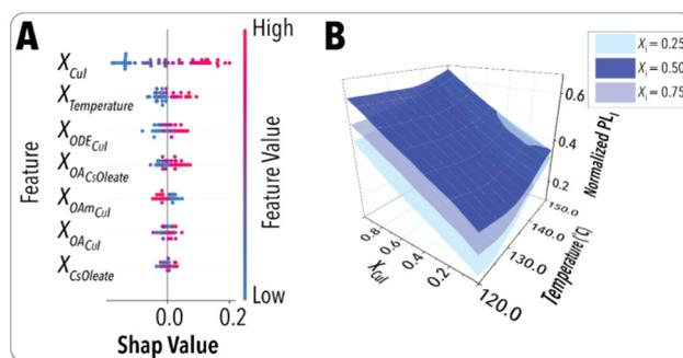
**Fig. 7** Accelerated fundamental studies of  $Cs_3Cu_2I_5$  NCs synthetic chemistry using the digital twin model: (A) Shapley additive explanation plot of  $PL_I$ . (B) Surface plot showing the impact of the top two synthesis input parameters on  $PL_I$ .
