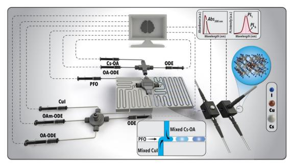
Fig. 2 Schematic illustration of the developed SDFL for fast-tracked synthesis and development of Pb-free MHP NCs.
