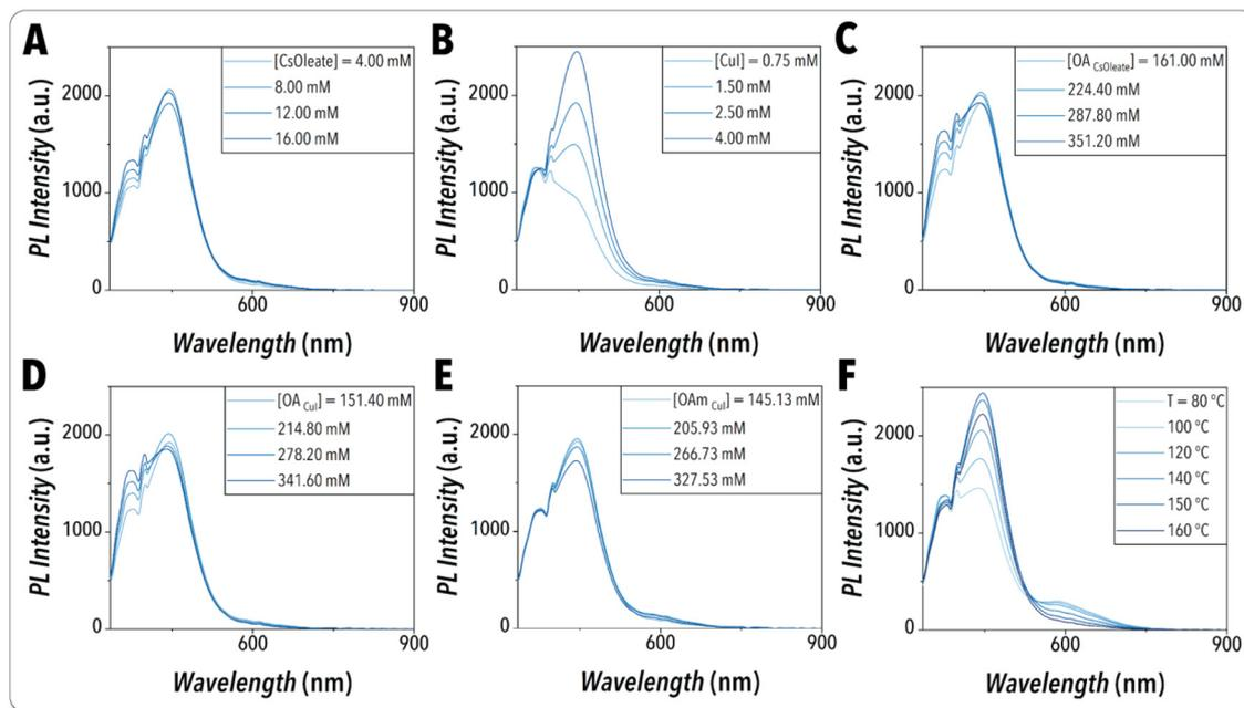
**Fig. 5** *In situ* recorded UV-Vis PL spectra of the partial grid search on the input synthesis parameters, including (A) [CsOleate], (B) [CuI], (C) [OAc<sub>CsOleate</sub>], (D) [OAm<sub>CuI</sub>], (E) [OAm<sub>CuI</sub>], and (F) reaction temperature, while maintaining the reaction time constant. The complete list of experimental conditions used for the partial grid search study is provided in Table S1.†
