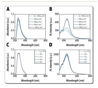
Fig. 4 In-flow screening for: the effect of total volumetric flowrate on the *in situ* recorded (A) absorption and (B) PL spectra while utilizing the same reaction time. The effect of reaction time on the *in situ* recorded (C) absorption and (D) PL spectra while utilizing total flowrates above 600 µL min<sup>-1</sup> to ensure the reaction mixing-independency.
