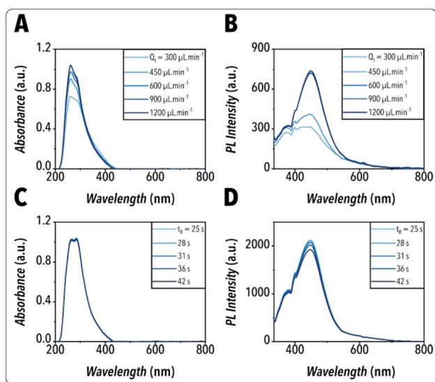
**Fig. 4** In-flow screening for: the effect of total volumetric flowrate on the *in situ* recorded (A) absorption and (B) PL spectra while utilizing the same reaction time. The effect of reaction time on the *in situ* recorded (C) absorption and (D) PL spectra while utilizing total flowrates above  $600\ \mu\text{L}\ \text{min}^{-1}$  to ensure the reaction mixing-independency.
