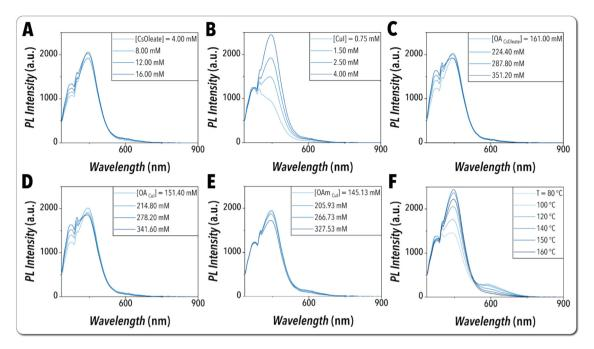
Fig. 5 In situ recorded UV-Vis PL spectra of the partial grid search on the input synthesis parameters, including (A) [CsOleate], (B) [CuI], (C) [OA<sub>CsOleate</sub>], (D) [OA<sub>Cul</sub>], (E) [OAm<sub>Cul</sub>], and (F) reaction temperature, while maintaining the reaction time constant. The complete list of experimental conditions used for the partial grid search study is provided in Table S1.†
