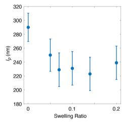
**Fig. 3** Persistence lengths of PMMA bottlebrush polymers in linear–bottlebrush hybrid systems at various swelling ratios of toluene (eqn (1)). The  $M_{\rm sc}$  of the bottlebrush polymer was 3500 g mol<sup>-1</sup>. Each data point consists of 350 chains. Error bars are the 90% confidence intervals, based on the 10 sets of 350 wormlike chains from simulations.
