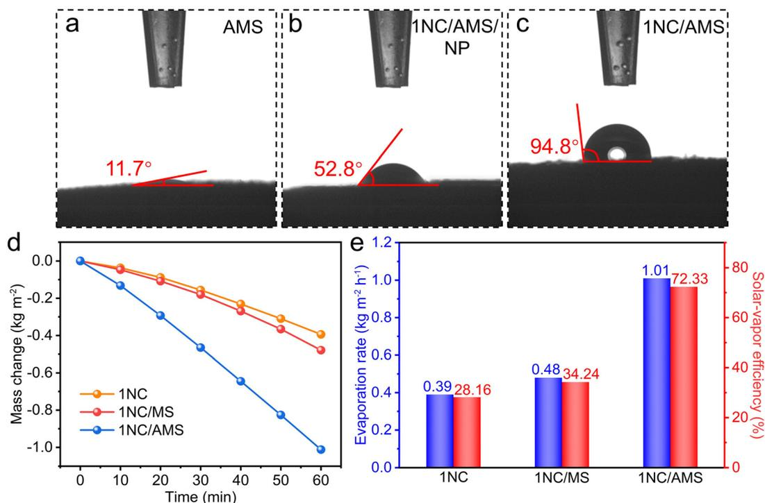
**Fig. 3** Water contact angle measurement over the (a) AMS, (b) 1NC/AMS/NP, and (c) 1NC/AMS. (d) Evaporation mass loss of 1NC, 1NC/MS and 1NC/AMS for 1 h under the simulated sunlight illumination (AM 1.5G) of one-sun intensity. (e) The average evaporation rates and the corresponding solar-vapor conversion efficiencies of 1NC, 1NC/MS and 1NC/AMS.
