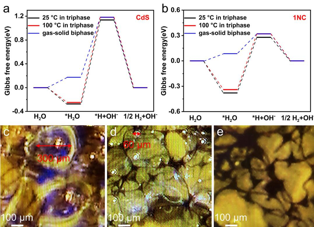
**Fig. 5** The calculated Gibbs free energy for the HER of the (a) CdS and (b) 1NC photocatalyst in the triphase system at different temperatures (25 and 100 °C), and in the gas–solid biphasic system. (c)–(e) Photographs of bubbles on the 1NC/AMS surface immersed at different depths below the liquid level of water observed under a microscope: (c) 5 mm, (d) 1 mm, (e) 0 mm. (The surface of 1NC/AMS is slightly higher than the liquid level of water.)
