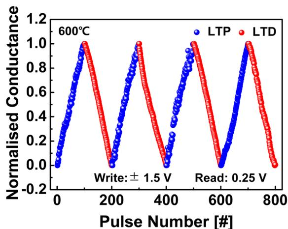
Fig. 10 Conductance saturation characteristics of HfO<sub>2</sub>/ZnO synaptic devices with thermal annealing at 600 °C under a series of positive pulses with different voltage amplitude.
