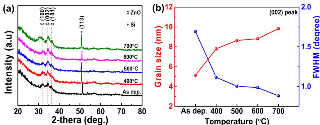
Fig. 3 (a) X-Ray diffraction spectra of HfO<sub>2</sub>/ZnO films without and with thermal annealing from 400 °C to 700 °C. (b) Dependence of the full width at half maximum (FWHM) and average grain size of HfO<sub>2</sub>/ZnO films on annealing temperature.
