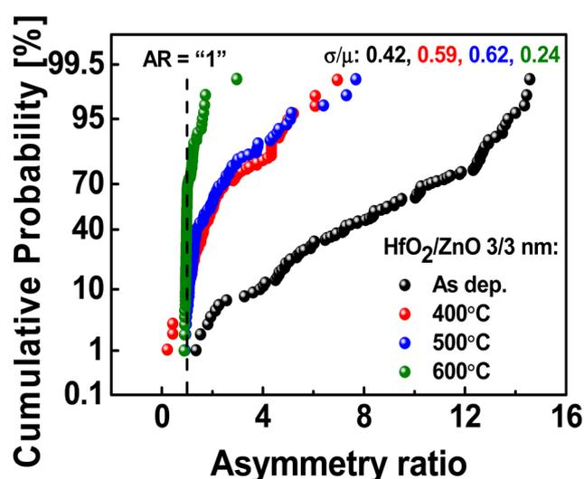
**Fig. 9** Cumulative probability of the asymmetry ratio for LTP and LTD behavior in bilayer  $\text{HfO}_2/\text{ZnO}$  synaptic devices without and with thermal annealing from 400 °C to 600 °C for 1 h in an  $\text{N}_2$  ambient, where the ratio “1” is the ideal state.
