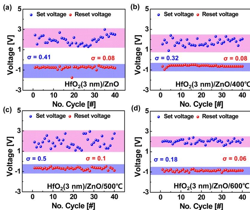
Fig. 6 Obtained VSET and VRESET distributions for 40 consecutive  $I$ – $V$  sweeps for bilayer  $\text{HfO}_2/\text{ZnO}$  synaptic devices (a) without and with thermal annealing at (b) 400 °C, (c) 500 °C, and (d) 600 °C.
