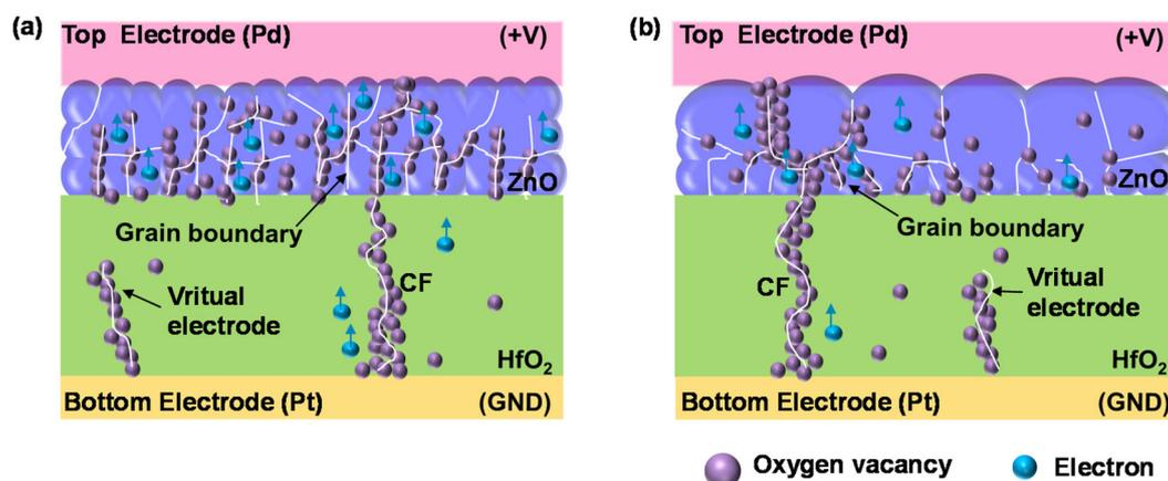
Fig. 11 Schematic illustration of the transition mechanism during the conductive filamentary formation in bilayer HfO<sub>2</sub>/ZnO synaptic devices (a) without and (b) with thermal annealing. Crystallized ZnO films formed by thermal annealing between the top Pd electrode and the HfO<sub>2</sub> layer remarkably improve O<sup>2-</sup> migration from the HfO<sub>2</sub> layer to the ZnO bulk and the top electrode interface.
