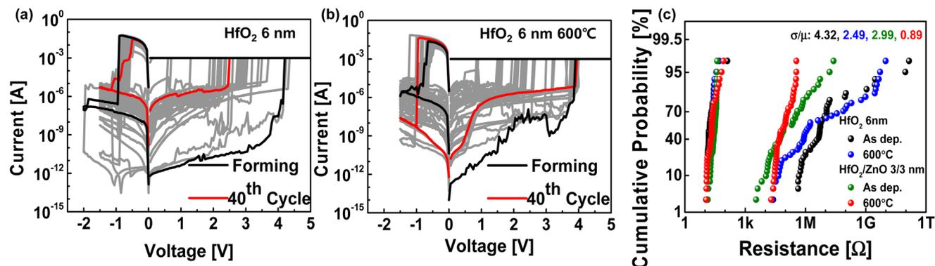
Fig. 7 Typical  $I$ - $V$  switching behavior of 6 nm HfO<sub>2</sub> (a) without and with thermal annealing (b) at 600 °C for 1 h in an N<sub>2</sub> ambient compared with that of bilayer HfO<sub>2</sub>/ZnO synaptic devices under the same thermal annealing conditions. (c) Distribution and cumulative probability of the HRS and LRS of HfO<sub>2</sub> (6 nm) and bilayer 3 nm HfO<sub>2</sub>/3 nm ZnO synaptic devices without and with thermal annealing.
