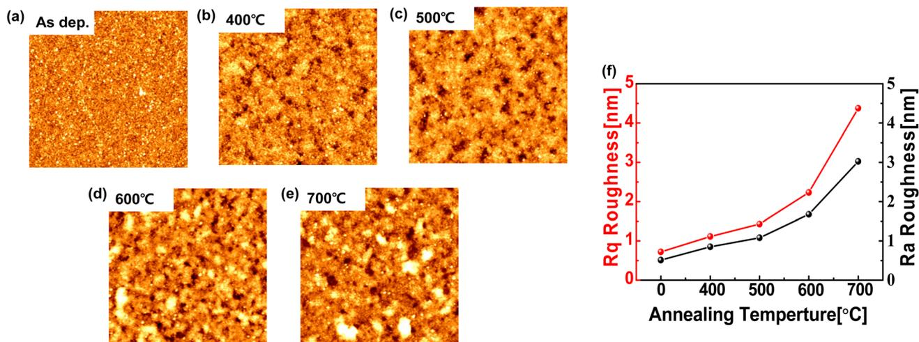
Fig. 2 AFM surface topography images of ZnO films in bilayer HfO<sub>2</sub>/ZnO synaptic devices (a) without thermal annealing, (b) with thermal annealing at 400 °C, (c) 500 °C, (d) 600 °C, and (e) 700 °C. (f) Dependence of the root mean square ( $R_q$  or  $R_{rms}$ ) and average roughness ( $R_a$ ) of ZnO films on thermal annealing.
