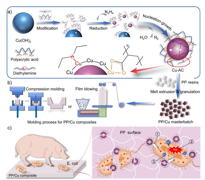
Fig. 1 Schematic illustrations of (a) the synthesis of surface-modified Cu nanoparticles and (b) melt blending for antibacterial masterbatches and their processing into composite films and sheets. (c) Schematic illustrations of the application of the polymeric antibacterial composite and its antibacterial mechanism
