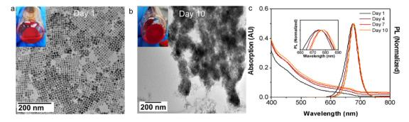
Fig. 5 TEM images and photos for the CsPbl<sub>3</sub> crude solution synthesised with Cs: Pb: I = 1:4:8 stoichiometry that is (a) as-synthesised, (b) stored for 10 days, and (c) evolution of corresponding UV-vis absorption and PL spectra with time (inset: zoom-in PL spectra showing the redshift of the PL peaks).
