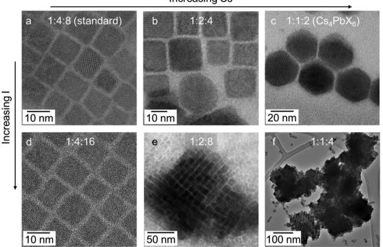
Fig. 2 TEM images of CsPbl<sub>3</sub> NCs synthesised using HDA-HI at different Cs: Pb: I molar ratios: (a) 1:4:8, (b) 1:2:4, (c) 1:1:2, (d) 1:4:16, (e) 1:2:8, and (f) 1:1:4. All images were taken immediately after synthesis.
