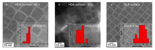
Fig. 3 TEM images and histograms for the measurement of the inter-NC surface distance for (a) HDA-Br capped NCs, (b) HDA-Br capped SCs, (c) OLA-Br capped NCs.
