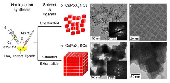
Fig. 1 (a) Schematic illustration of CsPbX<sub>3</sub> NC and SC syntheses. Structure illustration, low and high magnification TEM images for (b)-(d) CsPbI<sub>3</sub> NCs and (e-g) SCs. Insets of (c) and (f) are indexed SADP of NCs and SCs.
