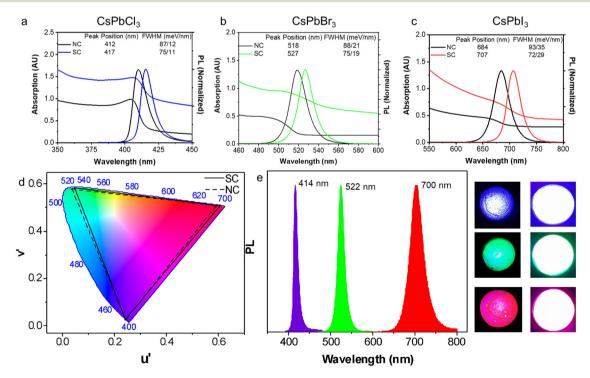
Fig. 6 UV-vis absorption and PL spectra for NC and SC films of (a) CsPbCl<sub>3</sub>, (b) CsPbBr<sub>3</sub> and (c) CsPbI<sub>3</sub>. (d) The emission of the NCs and SCs plotted on the colour gamut spectrum (CIE 1976); the PL is transformed into the UV through the chromaticity application in Origin software. (e) The PL spectra of the down-conversion LED devices fabricated from the SC-PMMA composites (left) and photos of the LEDs (right).
