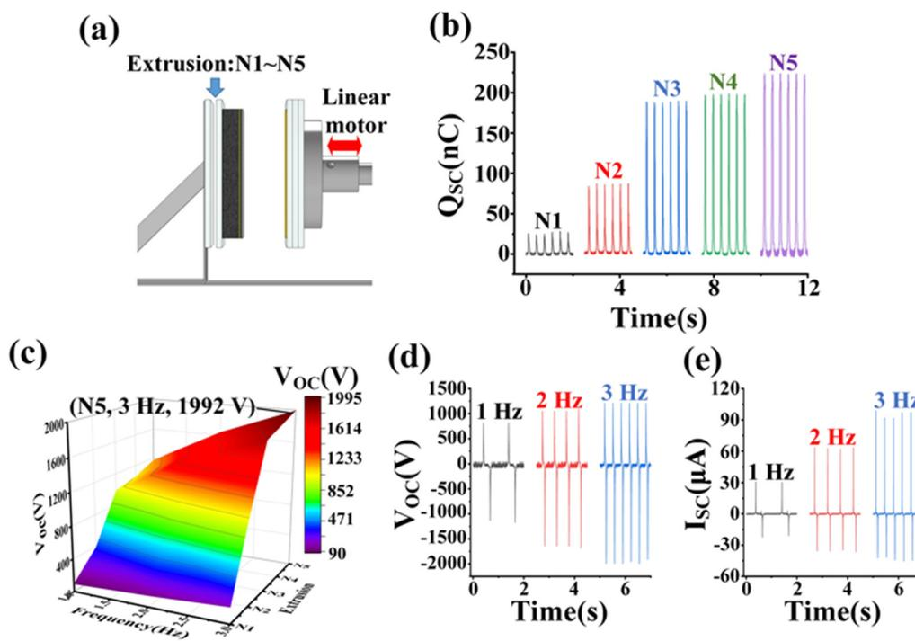
Fig. 3 (a) The working conditions of PFP-TENG. (b) The  $Q_{sc}$  values under different extrusion amounts. (c) The 3D surface graph of  $V_{oc}$  under different frequencies and extrusion amounts. The (d)  $V_{oc}$  and (e)  $I_{sc}$  changes at different frequencies.
