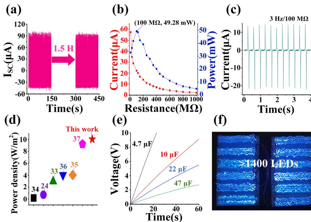
Fig. 4 (a) The reliability and (b) output power of PFP-TENG. (c) The output current at 100 M $\Omega$ . (d) Comparison of the power performance of PFP-TENG with previous designs. (e) The charging speed of difference capacitors using PFP-TENG. (f) The applicability of PFP-TENG in driving LEDs.
