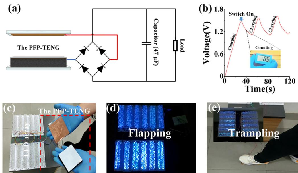
**Fig. 5** Application of PFP-TENG to drive low-power loads. (a) Using an external circuit drives (b) the electronic clock. (c) The PFP-TENG is applied in different motion occasions, such as (d) flapping and (e) trampling.
