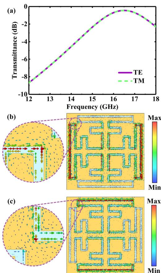
**Fig. 3** (a) Simulated transmittance of the MFSM in the Ku band (12–18 GHz) at normal incidence under TE and TM polarization. (b and c) Simulated surface current density of the MFSM at its resonant frequency (16.5 GHz) under (a) TE polarization and (b) TM polarization. Insets in (b) and (c) are the amplified surface current density of the corresponding purple dotted circle regions.
