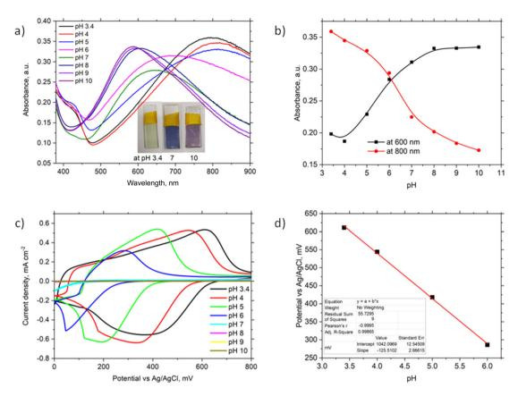
Fig. 3 Optical and electrochemical properties of ITO/PhNHPrSi/PANI: (a) UV-vis spectra of the monolayer by changing the buffer pH from 3.4 to 10 (inset: visualization of the samples after exposure to the buffer of pH 3.4, 7, and 10); (b) the pH and band maximum trends for protonation and deprotonation of the samples at 600 nm and 800 nm; (c) CVs of the electrodes by changing the buffer pH from 3.4 to 10; (d) the potential against pH plot.
