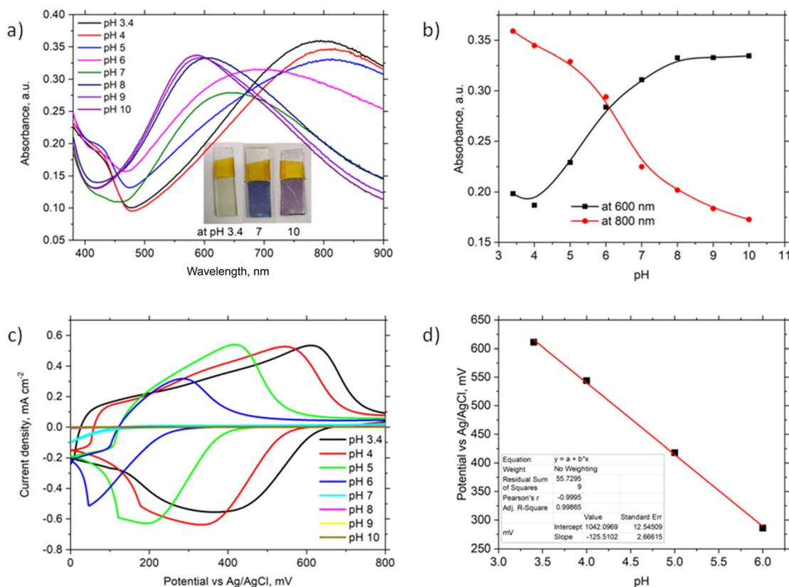
**Fig. 3** Optical and electrochemical properties of ITO/PhNHPrSi/PANI: (a) UV-vis spectra of the monolayer by changing the buffer pH from 3.4 to 10 (inset: visualization of the samples after exposure to the buffer of pH 3.4, 7, and 10); (b) the pH and band maximum trends for protonation and deprotonation of the samples at 600 nm and 800 nm; (c) CVs of the electrodes by changing the buffer pH from 3.4 to 10; (d) the potential against pH plot.
