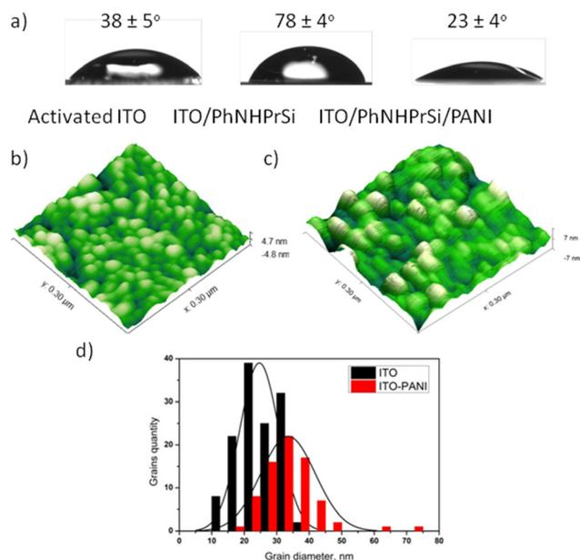
**Fig. 1** Properties of the ITO/PhNHPrSi/PANI surface: (a) the averaged water contact angles of the bare ITO, ITO/PhNHPrSi, and ITO/PhNHPrSi/PANI surfaces; (b) AFM image of the bare ITO and (c) the ITO/PhNHPrSi/PANI surfaces; (d) the statistical distributions of grain diameters (the histograms are mean distributions of the grains diameters) on the surfaces.
