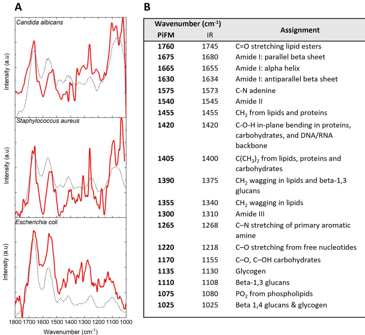
**Fig. 1** (A) Mean PiFM (red line) and FTIR spectra (black dotted line) for *E. coli*, *S. aureus* and *C. albicans* with reference spectra taken from the literature.<sup>50–52</sup> (B) Table comparing PiFM spectra against general FTIR assignments for microbial samples.
