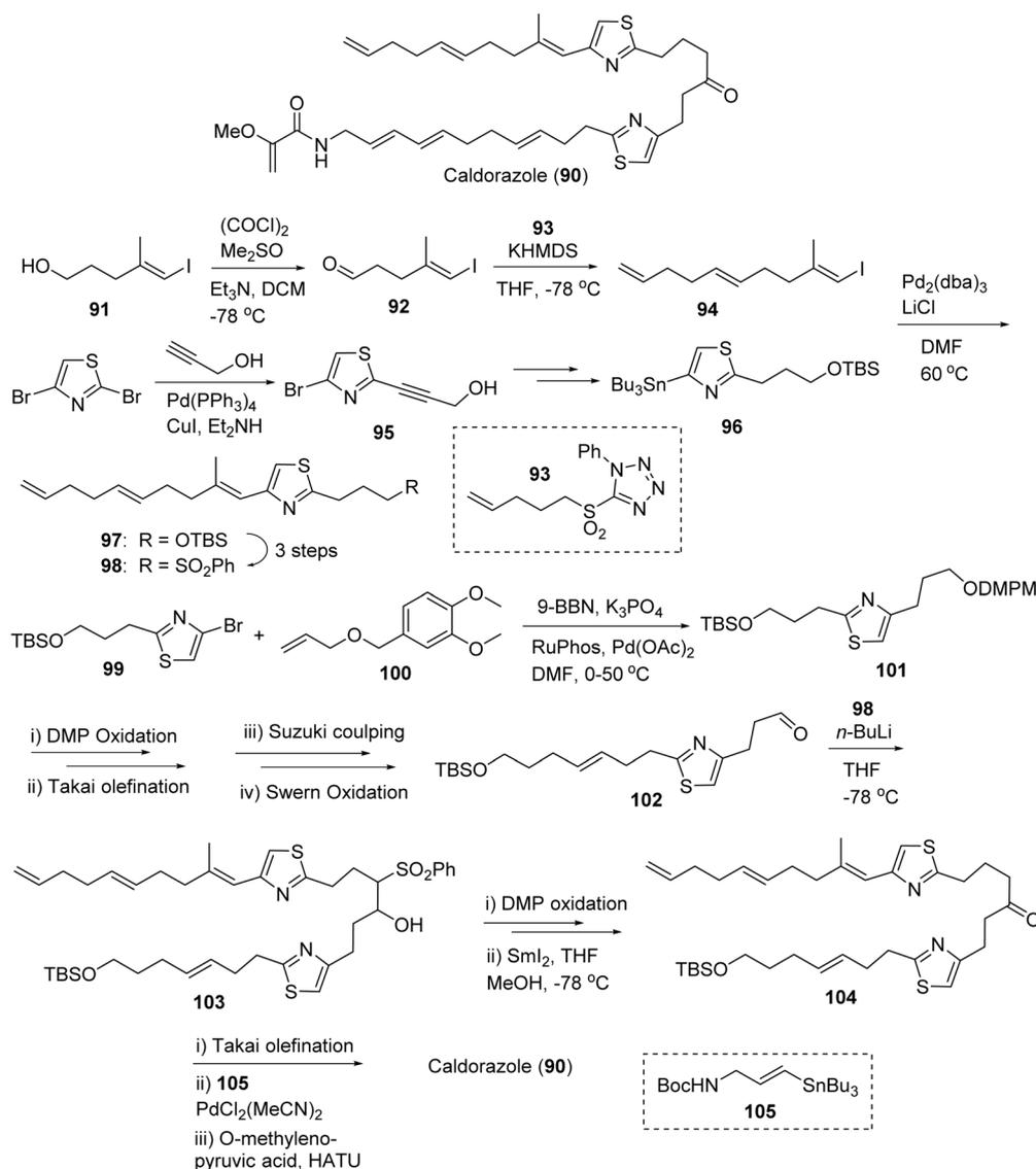
Fig. 23 Structures and total synthesis of caldorazole (90).
