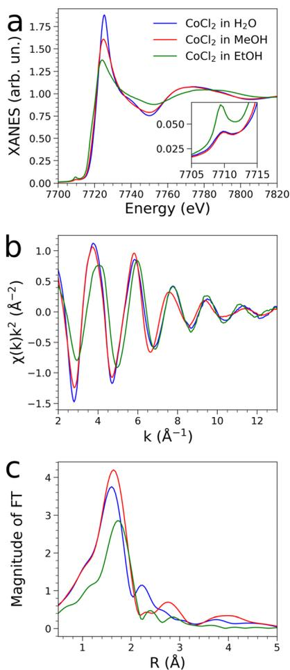
Fig. 2 Co K-edge (a) normalized XANES (inset: magnification of the pre-edge  $1s \rightarrow 3d$  transition), (b) EXAFS, and (c) non-phase shift-corrected FT experimental spectra collected on the  $0.1 \text{ mol L}^{-1}$   $\text{CoCl}_2$  aqueous, MeOH, and EtOH solutions.
