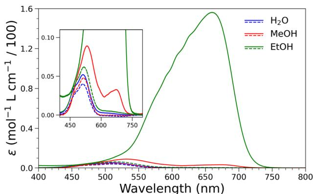
Fig. 1 Vis absorption spectra of the 0.1 mol L<sup>-1</sup>  $\text{CoCl}_2$  (full lines) and  $\text{Co}(\text{Tf}_2\text{N})_2$  (dashed lines) aqueous, MeOH, and EtOH solutions (inset: magnification of the 450–750 nm spectral region).
