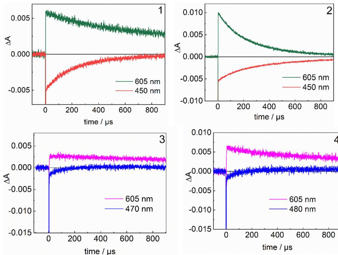
Fig. 5 Differential transient absorption kinetics at selected wavelengths in the presence of 20 mM  $\text{MV}^{2+}$  for the compounds studied in the  $\text{H}_2\text{O}/\text{CH}_3\text{CN}$  (4 : 1) argon-purged solution at 293 K. The solutions excited at 460 nm using a laser energy of  $\sim 10$  mJ and absorption at the excitation wavelength of 0.40.
