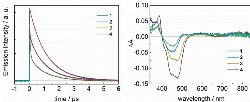
Fig. 4 Emission kinetics at the emission maximum (left) and transient absorption spectra at 100 ns (right) after the laser pulse, for the different compounds in  $\text{H}_2\text{O}/\text{CH}_3\text{CN}$  (4 : 1). Optically matched absorption at 460 nm. Decays have been fitted with a biexponential curve (red traces). On the right, the amplitude of the absorption spectra, taken at 100 ns after the laser pulse, is consistent with the excited state lifetimes.
