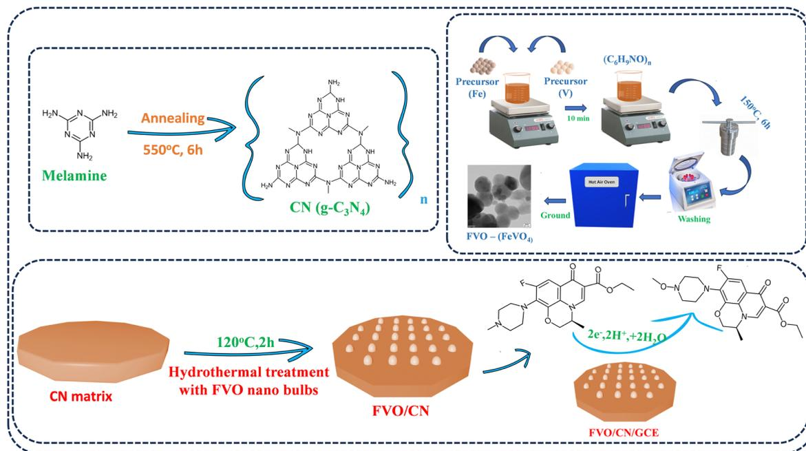
Scheme 1 Schematic representation demonstrating the synthesis of FVO/CN composite and its subsequent application in electrochemical sensing of LVO.
