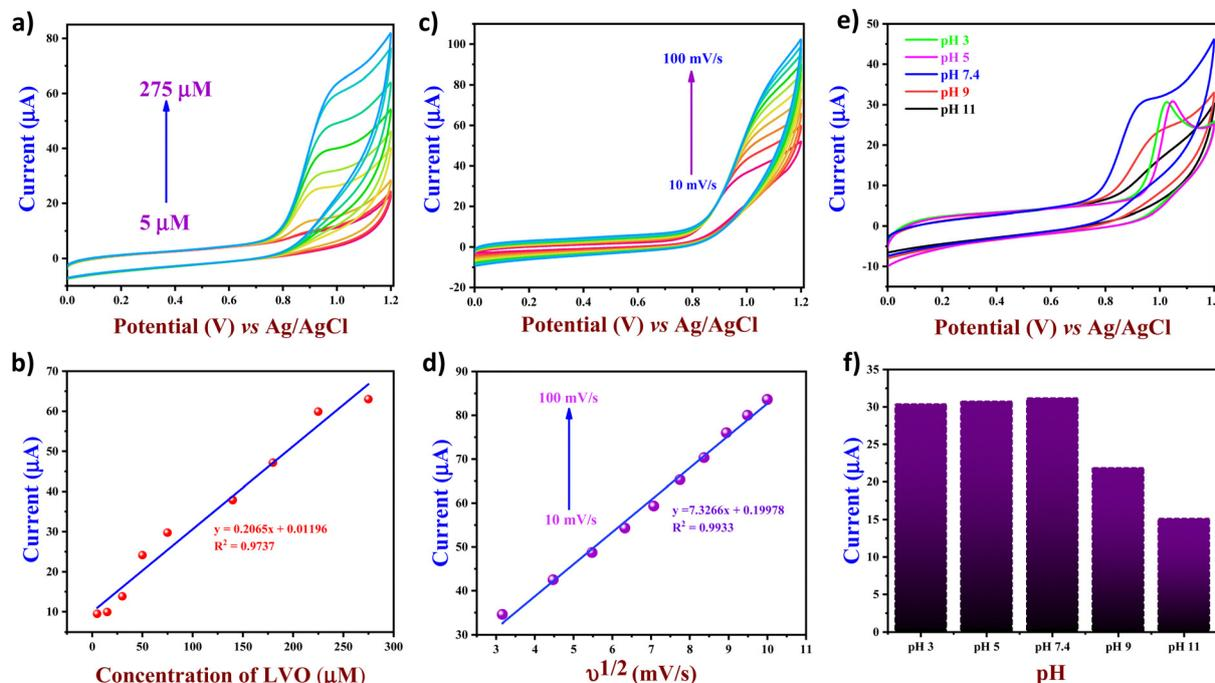
Fig. 6 (a) CV plots of FVO/CN/GCE with increasing concentration of LVO, (b) linear plot of peak current vs. the concentration of LVO, (c) CV plots of FVO/CN/GCE with increasing scan rates from 10 to 100  $\text{mV s}^{-1}$  in the presence of 250  $\mu\text{M}$  of LVO, (d) linear plot of peak current vs. square root of scan rates, (e) CV plots and (f) bar graph of current vs. pH of FVO/CN/GCE with various pH ranging from 3 to 11 with 120  $\mu\text{M}$  of LVO.
