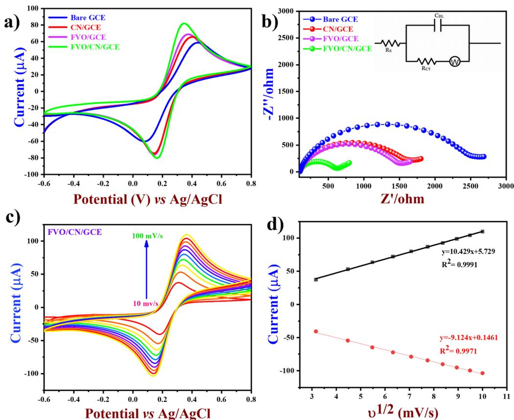
Fig. 4 (a) CV plots and (b) EIS plots of bare and different modified electrodes with 0.1 M KCl in 5 mM  $\text{Fe}(\text{CN})_6^{3-/4-}$ , (c) CV plots with increase in the scan rate from 10 to 100  $\text{mV s}^{-1}$  and (d) linear plots of  $I_{pa}$  and  $I_{pc}$  vs. square roots of scan rates of FVO/CN/GCE with 0.1 M KCl in 5 mM  $\text{Fe}(\text{CN})_6^{3-/4-}$ .
