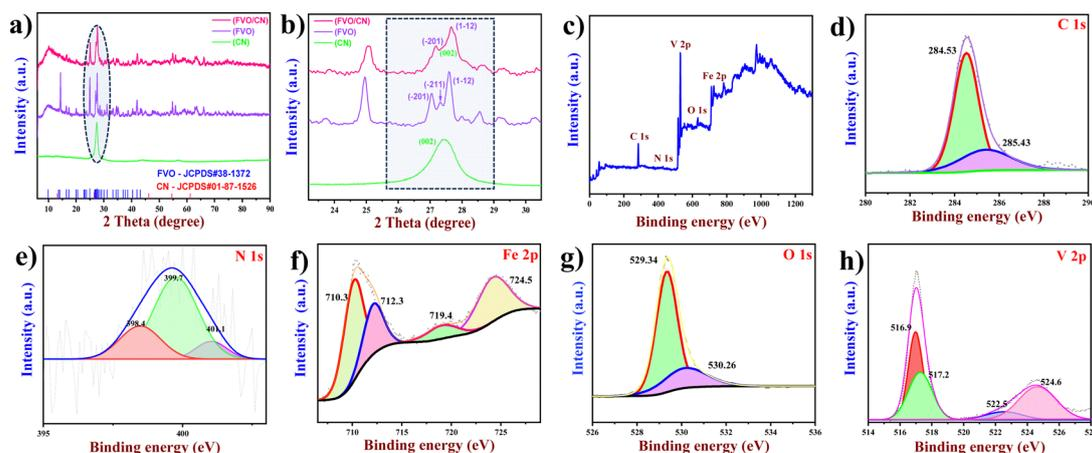
Fig. 1 (a) and (b) XRD patterns of CN, FVO and FVO/CN (c) XPS survey spectrum of FVO/CN, (d)–(h) deconvoluted spectrum of C 1s, N 1s, Fe 2p, and O 1s and the V 2p spectrum.
