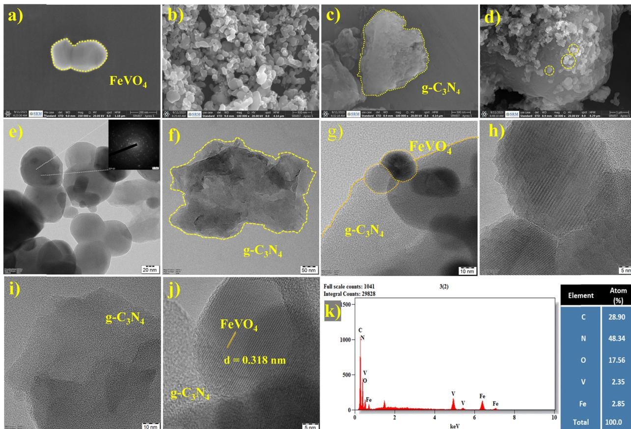
Fig. 3 SEM Micrographs of (a) and (b) FVO (FeVO<sub>4</sub>), (c) CN (g-C<sub>3</sub>N<sub>4</sub>), (d) FVO/CN, – TEM micrographs of (e)–(g) FVO, CN and FVO/CN, (h)–(j) lattice fringes of FVO, CN and FVO/CN, (k) EDX analysis of FVO/CN.
