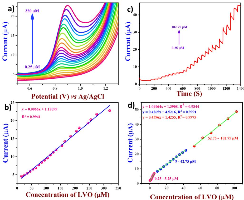
Fig. 7 (a) DPV curves of FVO/CN/GCE in 0.1 M PBS for LVO in the concentration range of 0.25–320  $\mu\text{M}$ , (b) linear plots of oxidation peak current vs. concentration of LVO, (c)  $i-t$  curve of FVO/CN/GCE was performed with the injection of different LVO concentrations (rotation rate = 1000 rpm and applied potential = +0.9 V) and (d) linear plots of current response vs. added LVO concentration.
