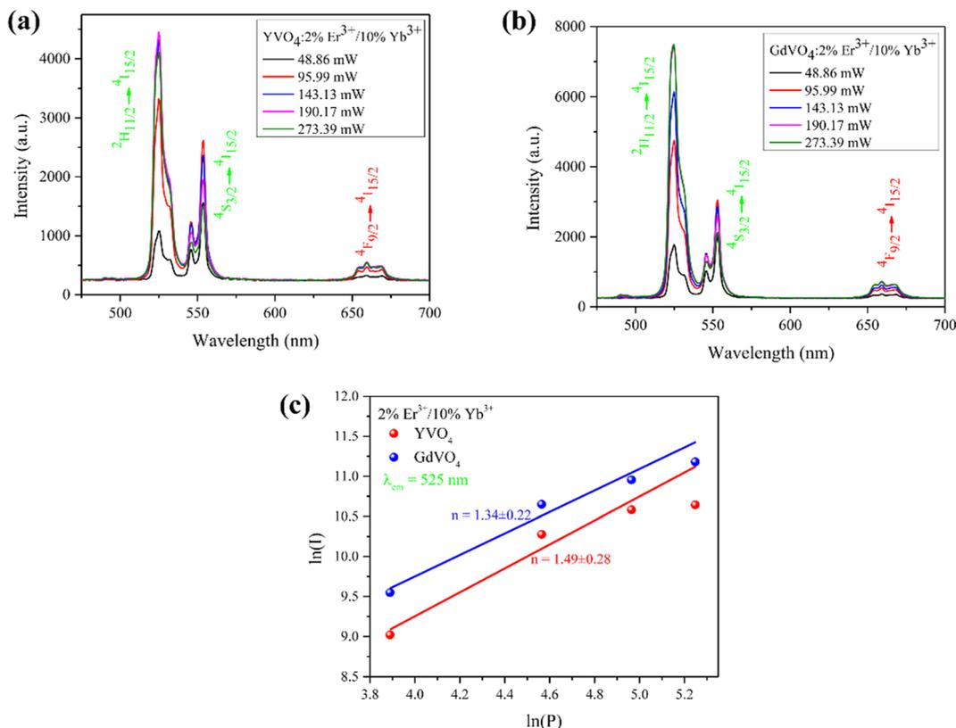
Fig. 8 Pump power-dependent UC emission spectra of Er<sup>3+</sup>/Yb<sup>3+</sup> co-doped (a) YVO<sub>4</sub> and (b) GdVO<sub>4</sub> and (c) ln(P)–ln(I) plot associated with the 525 nm emission.
