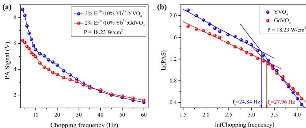
Fig. 9 (a) Variation of the photoacoustic signal amplitude with chopping frequency at an excitation power density of 18.23 W cm<sup>-2</sup> and (b) ln(chopping frequency)–ln(PAS) graph for transition frequency calculation.
