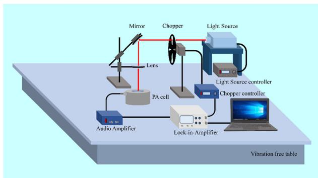
Fig. 2 Schematic diagram of a home-assembled photoacoustic spectrometer setup.
