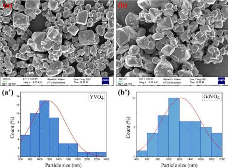
Fig. 4 (a) and (b) FE-SEM images and (a') and (b') particle size distribution of  $Er^{3+}/Yb^{3+}$  co-doped YVO<sub>4</sub> and GdVO<sub>4</sub>.
