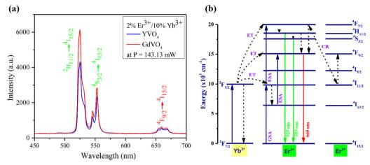
Fig. 7 (a) Upconversion emission spectra of  $Er^{3+}/Yb^{3+}$  co-doped [RE]VO<sub>4</sub>, (RE = Y, Gd) phosphors. (b) Energy level diagram and emission mechanisms of 980 nm excited Er3+ and Yb3+ ions.
