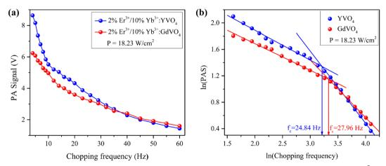
Fig. 9 (a) Variation of the photoacoustic signal amplitude with chopping frequency at an excitation power density of 18.23 W cm<sup>-2</sup> and (b) ln(chopping frequency)-In(PA signal) graph for transition frequency calculation.
