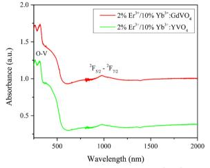
Fig. 6 UV-visible-NIR optical absorption spectra of  $Er^{3+}/Yb^{3+}$  co-doped GdVO<sub>4</sub> and YVO<sub>4</sub>.
