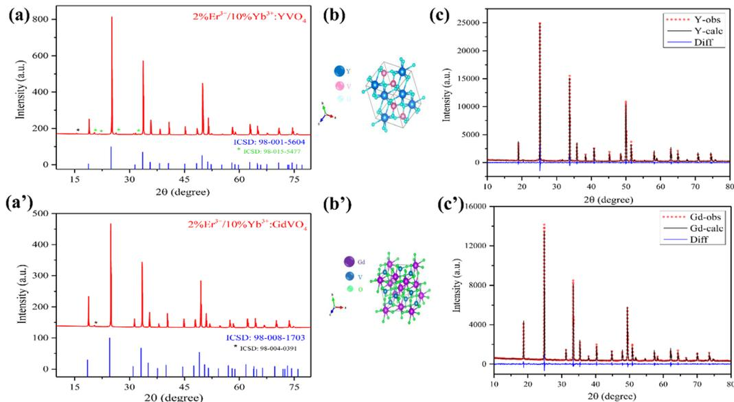
Fig. 3 (a and a') XRD pattern and (b and b') crystal structure of the unit cell and (c and c') Rietveld refinement of the XRD patterns of 2%Er<sup>3+</sup>/10%Yb<sup>3+</sup> co-doped YVO<sub>4</sub> and GdVO<sub>4</sub>.
