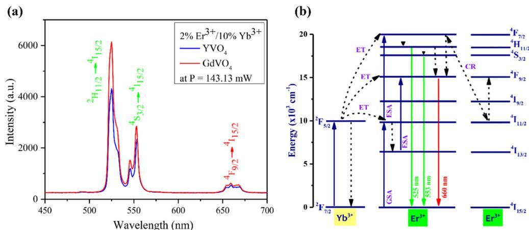
Fig. 7 (a) Upconversion emission spectra of  $\text{Er}^{3+}/\text{Yb}^{3+}$  co-doped  $[\text{RE}]\text{VO}_4$ , ( $\text{RE} = \text{Y}, \text{Gd}$ ) phosphors. (b) Energy level diagram and emission mechanisms of 980 nm excited  $\text{Er}^{3+}$  and  $\text{Yb}^{3+}$  ions.
