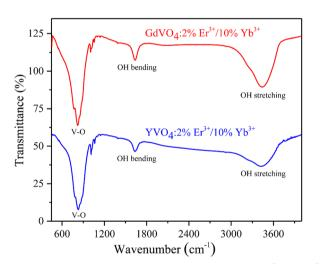
Fig. 5 Fourier-transform infrared spectroscopy (FTIR) of 2%Er<sup>3+</sup>/10%Yb<sup>3+</sup> co-doped YVO<sub>4</sub> and GdVO<sub>4</sub> phosphors.
