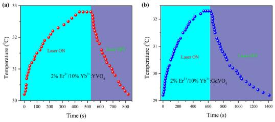
Fig. 10 Temperature variation with time under 980 nm laser irradiation of  $Er^{3+}/Yb^{3+}$  doped (a)  $YVO_4$  and (b)  $GdVO_4$
