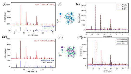
Fig. 3 (a and a') XRD pattern and (b and b') crystal structure of the unit cell and (c and c') Rietveld refinement of the XRD patterns of 2%Er<sup>3+</sup>/10%Yb<sup>3+</sup> codoped YVO<sub>4</sub> and GdVO<sub>4</sub>.
