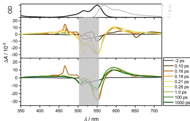
Fig. 7 Transient broadband absorption spectra of complex **4** in EtOH ( $\lambda_{\text{ex}} = 560$  nm, OD = 0.07). Probing between 350 and 720 nm was conducted at specified delay times (middle and bottom panels). A distinct grey area, located around 530 nm, is included in the figure to mask the spectral region affected by scattering effects from the excitation pulse. The top panel displays normalized steady-state absorption spectra (in black) and emission spectra (in grey).
