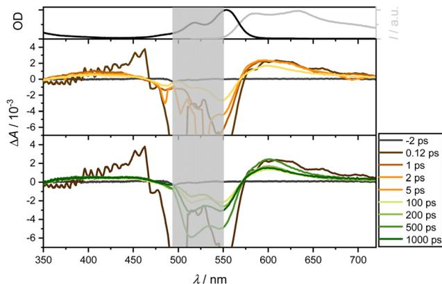
Fig. 6 Transient absorption spectra of **4** in DCM following excitation at 550 nm (OD = 0.21) and probing between 350 and 720 nm at specified delay times (middle and bottom panels). A distinct grey area, located around 530 nm, is included in the figure to mask the spectral region affected by scattering effects from the excitation pulse. Top: Normalized steady-state absorption spectra (black) and emission spectra (grey).
