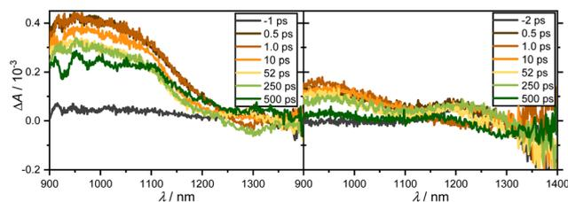
Fig. 8 Transient broadband absorption spectra of **3** (left, OD = 0.84) and **4** (right, OD = 1.03) in EtOH after excitation at 258 nm and probing between 900 and 1400 nm at the specified delay times.
