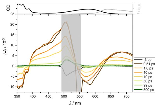
Fig. 4 Transient absorption spectra of the ligand **2** in DCM following excitation at 575 nm (OD = 0.2) were probed between 350 and 720 nm at the indicated delay times (bottom). A distinct grey area, located around 530 nm, is included in the figure to mask the spectral region affected by scattering effects from the excitation pulse. The top section shows the normalized steady-state absorption (black) and emission spectra ( $\lambda_{\text{ex}} = 500$  nm, slit width 4 nm, grey).
