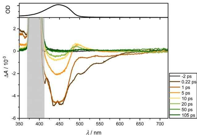
Fig. 5 Transient absorption spectra of ligand **1** in DCM following excitation at 400 nm (OD = 0.2) were recorded between 350 and 720 nm at the specified delay times (bottom). A distinct grey area, located around 400 nm, is included in the figure to mask the spectral region affected by scattering effects from the excitation pulse. The top section displays the normalized stationary absorption spectrum.
