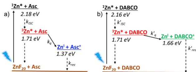
Fig. 6 Jablonski energy level diagram and reaction pathways for  $\text{ZnF}_{20}$  in the presence of (a) ascorbate and (b) DABCO as reversible electron donors.  $k_a = 1.5 (\pm 0.5) \times 10^6 \text{ M}^{-1} \text{ s}^{-1}$ ,  $k_{\text{rec}} = 1.3 (\pm 0.5) \times 10^8 \text{ M}^{-1} \text{ s}^{-1}$ ,  $k'_a = 9.2 (\pm 2.8) \times 10^7 \text{ M}^{-1} \text{ s}^{-1}$ ,  $k'_{\text{rec}} = 2.6 (\pm 0.8) \times 10^{10} \text{ M}^{-1} \text{ s}^{-1}$ .
