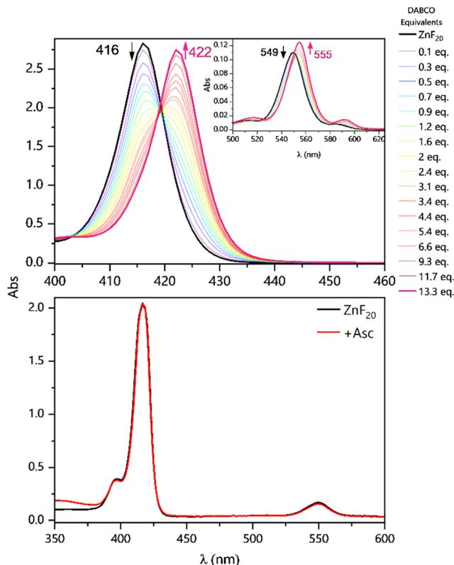
Fig. 2 Absorption changes in the Soret band region and in the Q-bands (inset) upon titration of 4.9  $\mu\text{M}$  ZnF<sub>20</sub> with DABCO (top panel) in CH<sub>3</sub>CN. Absorption spectrum of 4.9  $\mu\text{M}$  ZnF<sub>20</sub> in the absence and presence of 100 mM Asc (bottom panel) in CH<sub>3</sub>CN/H<sub>2</sub>O (6 : 4).
