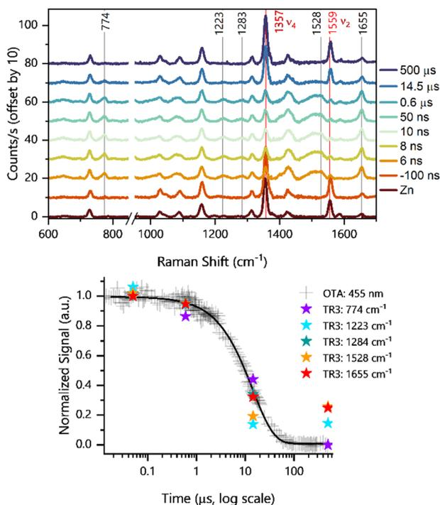
Fig. 4 TR3 spectra (top panel) obtained upon exciting  $12.6 \mu\text{M}$   $\text{ZnF}_{20}$  in  $\text{CH}_3\text{CN}$ . Solid vertical lines represent time-evolving bands due to the formation of  ${}^3\text{Zn}^*$ . Overlapped kinetic decays (bottom panel) obtained by OTA and TR3 under the same experimental conditions.  $\lambda_{\text{pump}} = 554 \text{ nm}$ , 2.2 mJ per pulse;  $\lambda_{\text{probe}} = 447 \text{ nm}$ , 2.2 mJ per pulse.
