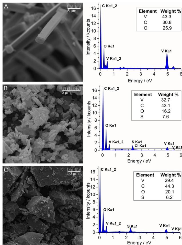
Fig. 3 Scanning electron microscopy (SEM) images at different magnifications (left) and EDS spectra (right) of: (A) crystalline **2,3-ampV**<sub>10</sub> × 10 000, (B) microcrystalline solid obtained from the direct reaction of an aqueous decavanadate solution with methylene blue (**MBV**<sub>10</sub>) × 15 000 and (C) amorphous solid obtained from the mixture of an aqueous decavanadate solution with toluidine blue (**TBV**<sub>10</sub>) × 1000.
