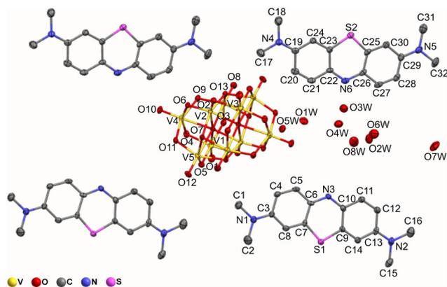
Fig. 4 Ellipsoid representation of  $[\text{MB}]_4[\text{H}_2\text{V}_{10}\text{O}_{28}] \cdot 10.8\text{H}_2\text{O}$ . Ellipsoids have been drawn at 30% probability. Hydrogen atoms of the MB cations have been omitted for clarity.
