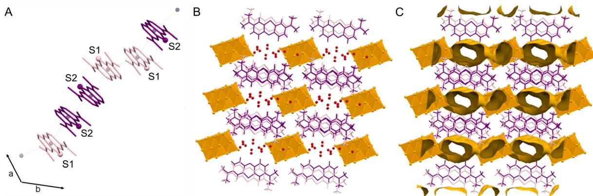
Fig. 5 (A) MB column along the  $c$  axis (B) crystal packing of **MBV<sub>10</sub>**, (C) voids in the crystal packing of **MBV<sub>10</sub>** (voids were calculated with the “voids” routine in mercury, probe radius = 1.2 Å, approx. grid spacings = 0.7 Å, voids are 19% of the unit cell volume).
