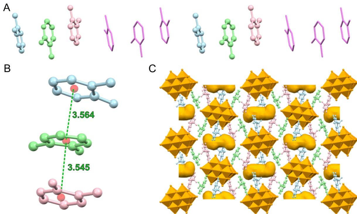
Fig. 2 (A) 2-Amino-3-methylpyridinium cation trimers viewed along the *a* axis (pink: the cation containing the N1 and N2 nitrogen atoms, light green: the cation containing the N3 and N4 nitrogen atoms, pale blue: the cation containing the N5 and N6 nitrogen atoms). (B) Disposition of the 2,3-ampH<sup>+</sup> trimers along the *c* axis. (C) Crystal packing of **2,3-ampV<sub>10</sub>** (with, in orange, the voids where the water molecules are located).
