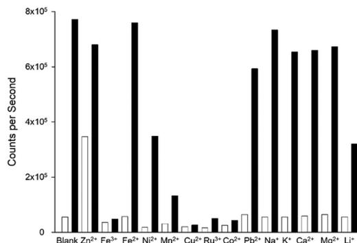
Fig. 10 Competition experiments for **P2**. The white bar represents **P2** (20  $\mu\text{M}$ , MeCN,  $\lambda_{\text{ex}}$  295 nm,  $\lambda_{\text{em}}$  465 nm) with 5.0 eq. of the indicated cation; the black bars is the same with 5.0 eq.  $\text{Cd}^{2+}$  after equilibrating for 3 min.
