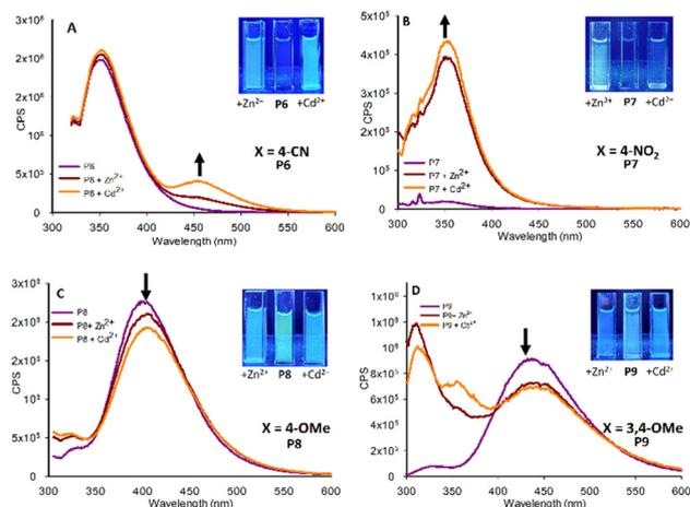
Fig. 6 Fluorescence studies of **P6–P9** (20  $\mu\text{M}$ , MeCN,  $\lambda_{\text{ex}}$  295 nm) with 5.0 eq.  $\text{Zn}^{2+}$  and  $\text{Cd}^{2+}$ , insets at  $\lambda_{\text{ex}}$  365 nm with the indicated metals, cps is counts per second.
