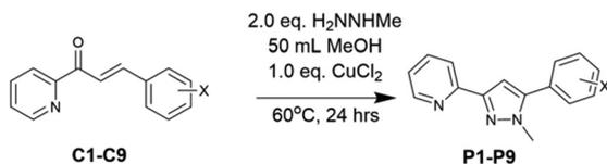
Scheme 4 Synthesis of **P1–P9** using optimised conditions.
