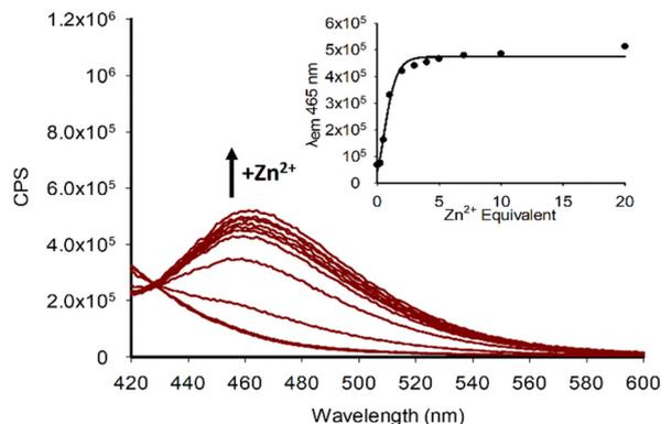
Fig. 7 Fluorescence studies of **P2** (20  $\mu\text{M}$ , MeCN,  $\lambda_{\text{ex}}$  295 nm) with increasing eq. of  $\text{Zn}^{2+}$  0.125, 0.25, 0.50, 1.0, 2.0, 3.0, 4.0, 5.0, 7.0, 10.0 and 20.0 eq. Inset is  $\lambda_{\text{em}}$  at 465 nm, cps is counts per second.
