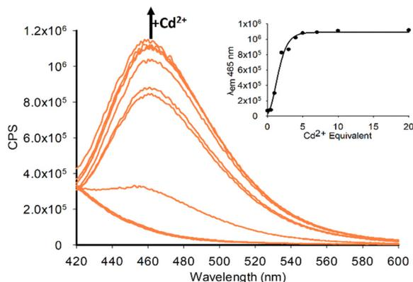
Fig. 8 Fluorescence studies of **P2** (20  $\mu\text{M}$ , MeCN,  $\lambda_{\text{ex}}$  295 nm) with increasing eq. of  $\text{Cd}^{2+}$  0.125, 0.25, 0.50, 1.0, 2.0, 3.0, 4.0, 5.0, 7.0, 10.0 and 20.0 eq. Inset is  $\lambda_{\text{em}}$  at 465 nm, cps is counts per second.
