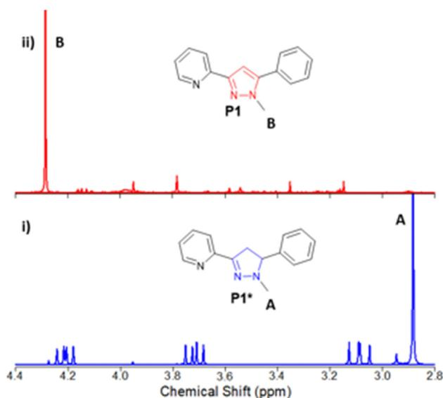
Fig. 2 Representative example of <sup>1</sup>H NMR study to determine the % conversion of methyl group A in **P1\*** (in blue, entry 18, Table 2, i) to methyl group B in **P1** (in red, entry 19, Table 2, ii).
