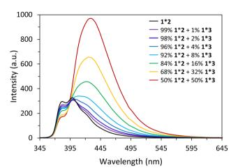
Fig. 4 Fluorescence measurements of self-assembled nanostructures at 20 °C: **1\*2** (black) and **1\*3** doped spheres with 99–50% **1\*2** and 1–50% **1\*3** (coloured). Fluorescence quantum yields can be found in Fig. S19 ESI.‡ Conditions: 1  $\mu$ M **1**, 1–0.5  $\mu$ M **2**, 0–0.5  $\mu$ M **3**, 10 mM sodium phosphate buffer pH 7.2, 0.10 mM spermine tetrahydrochloride, 20 vol% ethanol,  $\lambda_{ex}$  330 nm.
