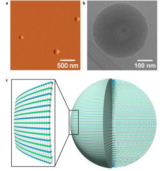
Fig. 3 (a) AFM deflection image of 1\*2 deposited on APTES-modified mica, (b) cryo-EM image of 1\*2, and (c) illustration of a self-assembled 1\*2 nanosphere and zoom-in on outermost layer (DNA in grey, 2,7-dialkynyl phenanthrene **2,7-Ph** in blue, and **3**,6-dialkynyl phenanthrene  $\alpha$  in green). Conditions: 1 µM 1\*2, 10 mM sodium phosphate buffer pH 7.2, 0.10 mM spermine tetrahydrochloride, and 20 vol% ethanol.
