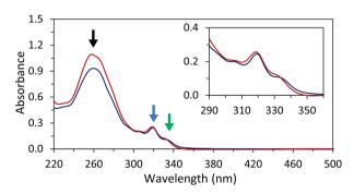
Fig. 2 Temperature-dependent UV-vis absorption spectra of disassembled 1\*2 at 75 °C (red) and self-assembled 1\*2 at 20 °C (blue). Highlighted by arrows: absorption of DNA nucleobases, 3,6- and 2,7dialkynyl phenanthrene (black), 3,6- and 2,7-dialkynyl phenanthrene absorption (blue), and 3,6-dialkynyl phenanthrene (green). Conditions: 1 μM 1\*2, 10 mM sodium phosphate buffer pH 7.2, 0.10 mM spermine tetrahydrochloride, 20 vol% ethanol.
