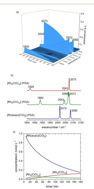
Fig. 4 (a) In situ FTIR-spectra series obtained from the treatment of [Rh(acac)(CO)<sub>2</sub>] with synthesis gas at  $\nu$  = 100 °C. Conditions: [Rh] = 1 mM,  $p(CO/H_2) = 2.0$  MPa, solvent: n-dodecane; (b) extracted PGAspectra; (c) concentration profiles after scaling based on calibration data.
