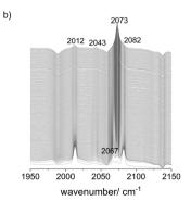
Fig. 12 In situ FTIR spectra collected during the hydroformylation of neohexene covering the first 15 min (a) and the entire conversion range (b). Conditions: [Rh] = 1 mM, [alkene] = 1 M,  $\nu$  = 90 °C, p(Ar) = 0.5 MPa,  $p(CO/H_2) = 2.0$  MPa, solvent: cyclohexane
