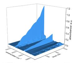
Fig. 1 In situ FTIR-spectra collected during the perturbation experiment monitoring the decomposition of [Rh(acac)(CO)<sub>2</sub>] under syngas atmosphere. Conditions: [Rh] = 0.5–10 mM, [DPC] = 2 mM,  $\nu$  = 120 °C, p(CO/  $H_2$ ) = 2.0 MPa, solvent: n-dodecane.
