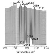
Fig. 9 In situ FTIR spectra collected during the treatment of  $[Rh_4(CO)_{12}]$ , preformed from [Rh(acac)(CO)<sub>2</sub>], with ethene in the presence of synthesis gas. Conditions: [Rh] = 1 mM,  $p(CO/H_2)$  = 2.0 MPa,  $p(C_2H_4)$  = 1.0 MPa,  $\nu$  = 30 °C, solvent: n-dodecane
