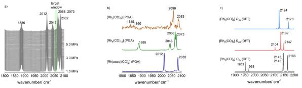
Fig. 8 (a) In situ FTIR spectra collected during the CO partial pressure variation (1.0 – 5.0 MPa) to populate [Rh<sub>2</sub>(CO)<sub>8</sub>]. Conditions: [Rh] = 1 mM,  $\nu$  = 30 °C, solvent: n-dodecane; (b) PGA spectra for [Rh2(CO)8], [Rh4(CO)12] and [Rh(acac)(CO)2] based on the entire IR-spectroscopic data including formation of  $[Rh_4(CO)_{12}]$  from  $[Rh(acac)(CO)_2]$ ; (c) calculated vibrational spectra for isomeric forms of  $[Rh_2(CO)_8]$  via DFT methods
