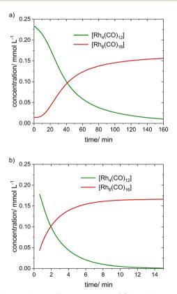
Fig. 5 Concentration profiles extracted via PGA and linear regression from in situ FTIR-spectra collected during treatment of [Rh<sub>4</sub>(CO)<sub>12</sub>] under (a) synthesis gas  $p(CO/H_2) = 2.0$  MPa and (b) argon p(Ar) = 0.1 MPa. Further conditions: [Rh] = 1 mM,  $\nu$  = 100 °C, solvent: n-dodecane
