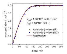
Fig. 11 Hydroformylation of neohexene. Concentration-time data for the product aldehyde formation (n + iso). Fitted numerical integration/regression data based on the rate equation:  $V = V_{sat}[S]/(K_m + [S])$ . Conditions: [Rh] = 1 mM, [alkene] = 1 M,  $\nu$  = 90 °C, p(Ar) = 0.5 MPa,  $p(CO/H_2)$  = 2.0 MPa, t = 6 h, solvent: cyclohexane.
