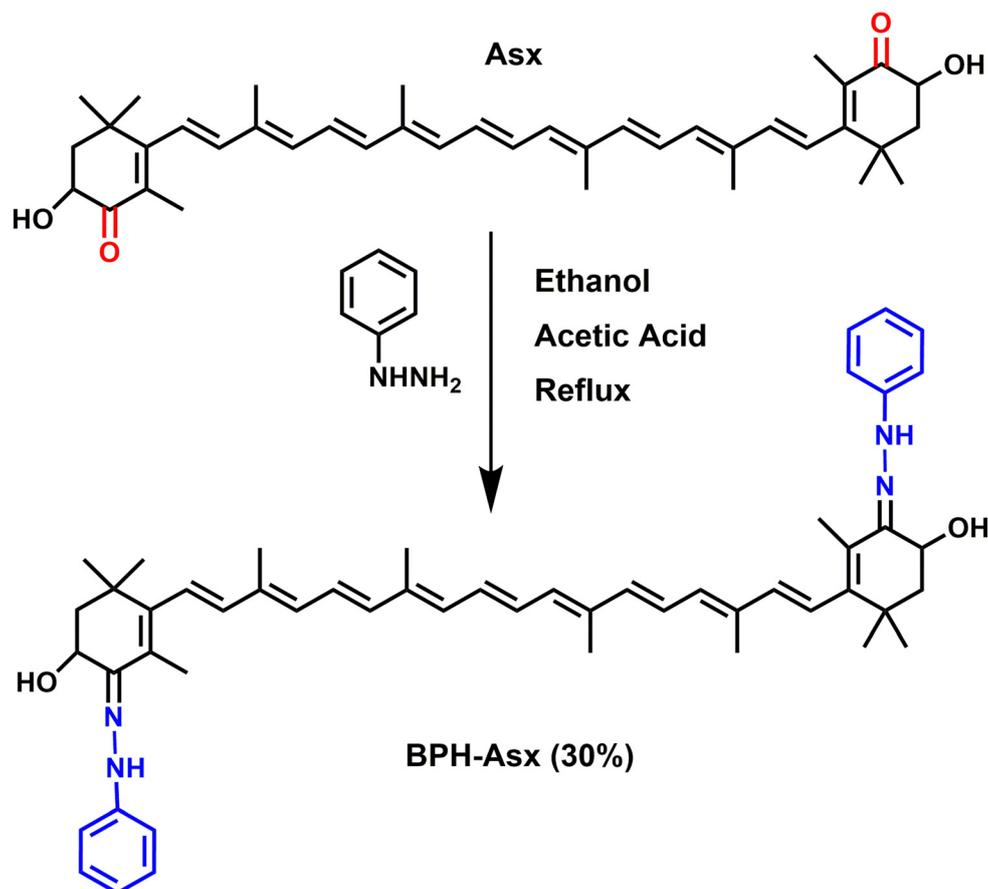
Scheme 1 Synthetic pathway of bis-phenylhydrazone astaxanthin (BPH-Asx).
