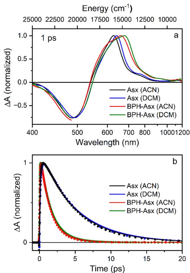
Fig. 3 (a) Normalized transient absorption spectra of **Asx** and **BPH-Asx** in both solvents. The spectra were measured at 1 ps after excitation at 500 nm for all compounds/solvents. (b) Normalized kinetics measured at the  $S_1$ - $S_n$  maximum for each sample. The solid lines represent fits obtained from global fitting analysis.
