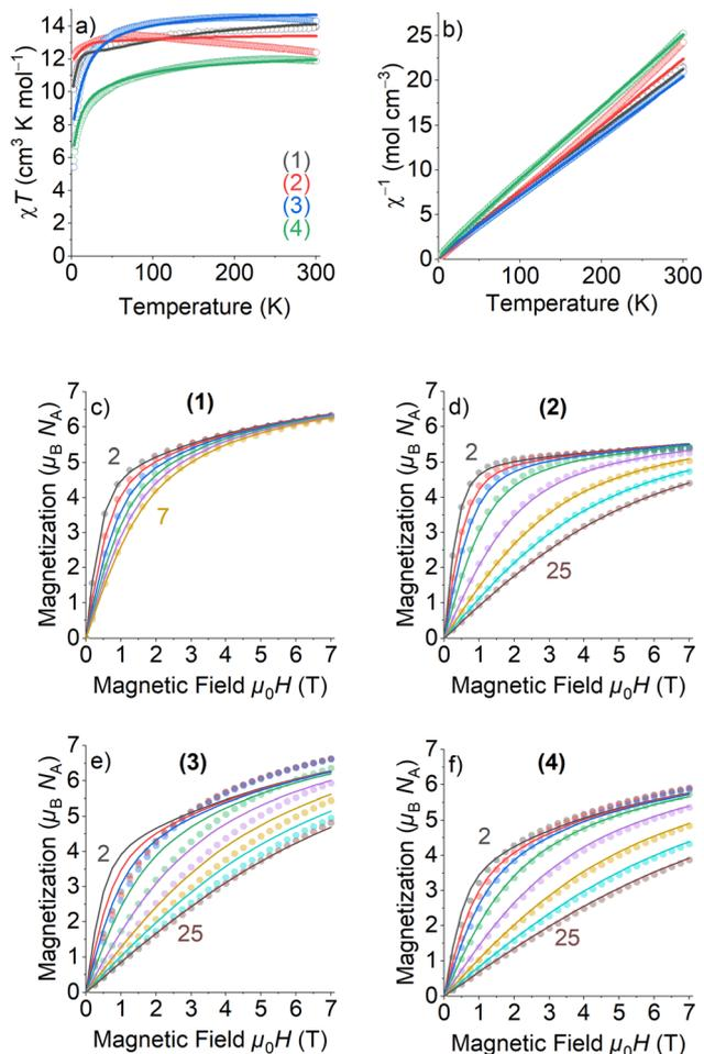
Fig. 4 DC magnetometry measurements (circles) and fits of magnetic models (lines) obtained for **1–4**: (a)  $\chi T$  vs. temperature, (b) inverse susceptibility  $\chi^{-1}$ , and (c)–(f) magnetization vs. field. The numbers give the lowest and highest temperatures in K, respectively, of the measured field scans.
