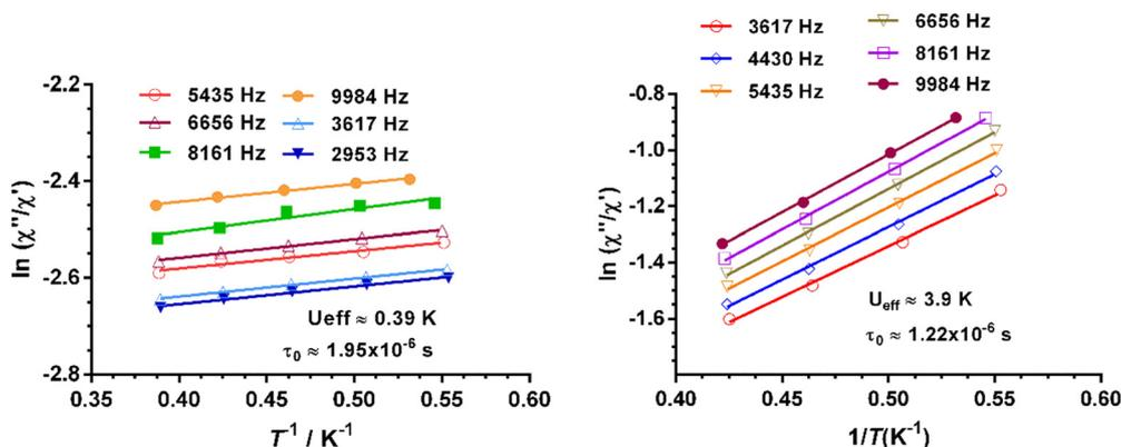
Fig. 5 Temperature dependence of the  $\ln(\chi''_M/\chi'_M)$  at different frequencies under a magnetic field of zero (left) and 588 Oe for **1**. Solid lines correspond to the fit of the experimental data to eqn (2).
