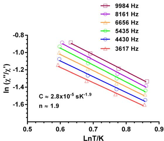
Fig. 6 Dependence of the ratio of the  $\ln(\chi''_M/\chi'_M)$  with  $\ln T$  at different frequencies under a magnetic field of 588 Oe for 1. Solid lines correspond to the fit of the experimental data to eqn (3).
