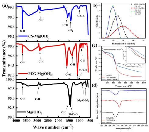
Fig. 4 (a) FTIR, (b) DLS, and (c) TGA profile of bare MHNPs, PEG, and chitosan-coated MHNPs, and (d) first TGA derivative weight loss percentage of MHNPs
