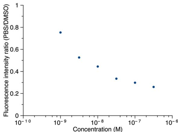
Fig. 8 The ratio of the fluorescence intensity of **1'** in PBS versus DMSO as a function of concentration. In DMSO,  $\lambda_{\text{abs}} = 419 \text{ nm}$ ,  $\lambda_{\text{em}} = 641 \text{ nm}$ ; in PBS,  $\lambda_{\text{abs}} = 415 \text{ nm}$ ,  $\lambda_{\text{em}} = 645 \text{ nm}$ .
