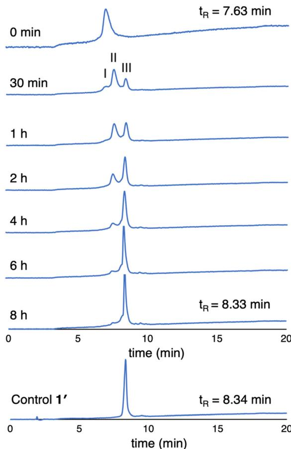
Fig. 6 RP-HPLC traces ( $\lambda_{\text{abs}} 420 \text{ nm}$ ) monitoring dephosphorylation of **1** upon treatment with ALP over 8 hours ( $100 \mu\text{M}$ ,  $2 \text{ U mL}^{-1}$  ALP). The trace at 0 min is prior to treatment with ALP.
