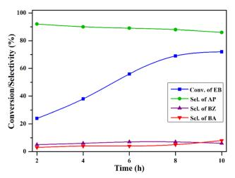
Fig. 12 The influence of the reaction time on oxidation of ethylbenzene. Reaction conditions: ethylbenzene (25 mL), temperature (120 °C), O<sub>2</sub> pressure (20 bar), and catalyst (50 mg).
