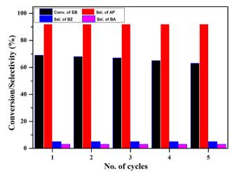
Fig. 14 Reusability study. Reaction conditions: ethylbenzene (25 mL). temperature (120 °C), O<sub>2</sub> pressure (20 bar), catalyst (50 mg), and time (8 h).
