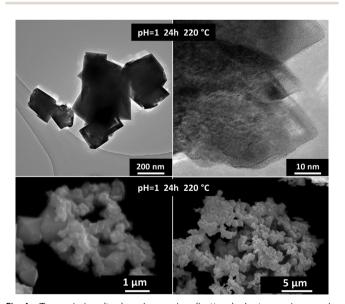
Fig. 1 Transmission (top) and scanning (bottom) electron micrographs of CeO<sub>2</sub> powder obtained by the hydrothermal decomposition of  $Ce_2(C_2O_4)_3\cdot 10H_2O$  in nitric acid solution (pH = 1) at 220 °C for 24 h.
