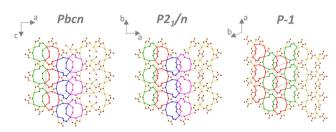
Fig. 5 Structural motifs of oxalate layers perpendicular to the infinite coordination polymer chains. Coordinated water molecules (except those forming the oxalate layer and water in pores) have been omitted for clarity.
