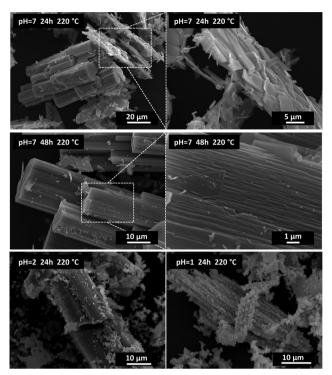
Fig. 2 Scanning electron micrographs of cerium oxalate with different degrees of conversion to CeO<sub>2</sub>. Assemblies of the recrystallised phase with initial  $Ce_2(C_2O_4)_3$ :10H<sub>2</sub>O (top), recrystallisation and change of morphology to rods (middle), and disintegration of the rods to nanocrystalline CeO<sub>2</sub>
