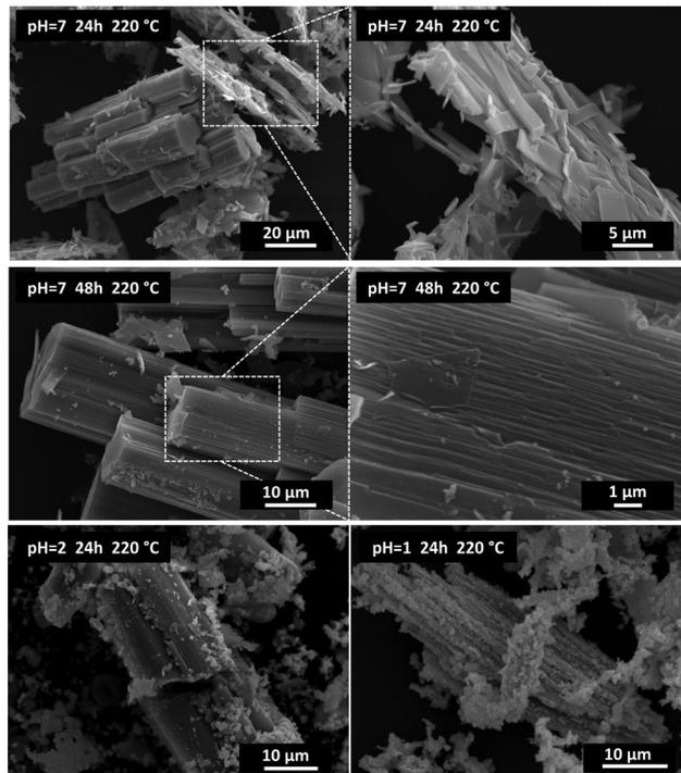
Fig. 2 Scanning electron micrographs of cerium oxalate with different degrees of conversion to  $\text{CeO}_2$ . Assemblies of the recrystallised phase with initial  $\text{Ce}_2(\text{C}_2\text{O}_4)_3 \cdot 10\text{H}_2\text{O}$  (top), recrystallisation and change of morphology to rods (middle), and disintegration of the rods to nanocrystalline  $\text{CeO}_2$  (bottom).
