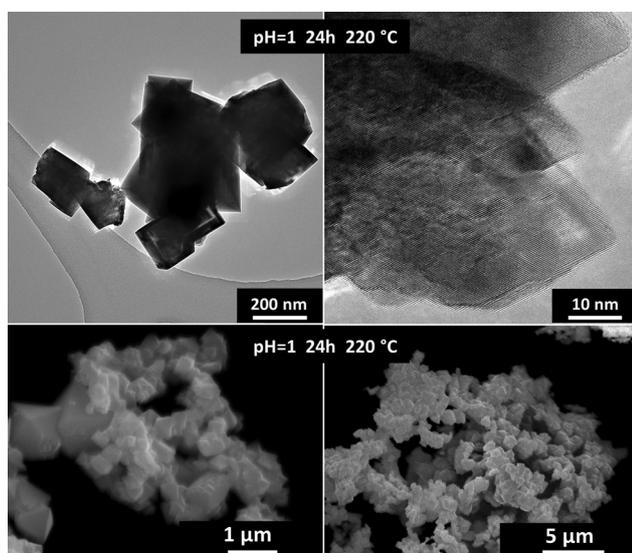
Fig. 1 Transmission (top) and scanning (bottom) electron micrographs of  $\text{CeO}_2$  powder obtained by the hydrothermal decomposition of  $\text{Ce}_2(\text{C}_2\text{O}_4)_3 \cdot 10\text{H}_2\text{O}$  in nitric acid solution (pH = 1) at 220 °C for 24 h.
