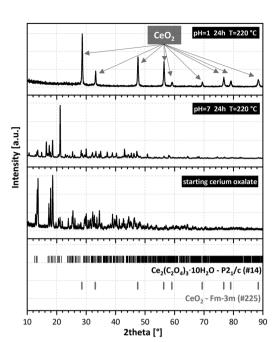
Fig. 3 Powder X-ray diffraction of the initial Ce<sub>2</sub>(C<sub>2</sub>O<sub>4</sub>)<sub>3</sub>·10H<sub>2</sub>O (bottom), hydrothermally treated (middle), and final CeO<sub>2</sub> (top)
