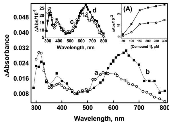
Fig. 2 Transient absorption spectra generated from pulse radiolysis of N<sub>2</sub>O-saturated solution containing compound **1** (50 μM) in water (a = 2 μs, b = 10 μs) and in the presence of 5 mM phosphate buffer at pH 7 (c = 2 μs, d = 10 μs). Inset (A) shows the variation of absorbance at 630 nm (■) and 380 nm (○) as a function of the concentration of **1**.
