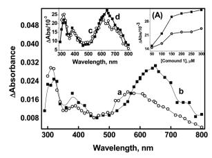
Fig. 2 Transient absorption spectra generated from pulse radiolysis of  $N_2$ O-saturated solution containing compound **1** (50  $\mu$ M) in water ( $a = 2 \mu s$ ,  $b = 10 \mu s$ ) and in the presence of 5 mM phosphate buffer at pH 7 ( $c = 2 \mu s$ ,  $d = 10 \mu s$ ). Inset (A) shows the variation of absorbance at 630 nm ( $\blacksquare$ ) and 380 nm (○) as a function of the concentration of 1.
