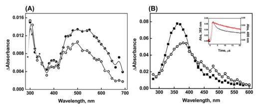
Fig. 5 Transient absorption spectra obtained on reaction between 100  $\mu$ M compound 2 and (A)  $CO_3^{\bullet}(O) = 4 \mu$ S,  $O(O) = 20 \mu$ S) and (B)  $O(O) = 20 \mu$ S) and (B) an 2  $\mu$ s,  $O = 5 \mu$ s) at pH 7. The inset in plot (B) is the absorbance-time plot obtained on reaction of compound 2 with Br<sub>2</sub>  $^{\bullet}$  radical (black line = 365 nm, red line = 400 nm).
