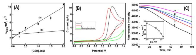
Fig. 6 Plot (A) is the observed decay rate of the radical cation with varying concentrations of GSH, where (a) corresponds to compound 1 and (b) corresponds to compound 2. Plot (B) is the cyclic voltammogram of compound 1 and 2 in phosphate buffer at pH 7. Plot (C) shows the decay of fluorescein due to degradation by peroxyl radical in the absence (trace a) and in the presence of compound 2 (b = 0.5 mM, c = 0.7 mM, d = 0.8 mM and e = 0.9 mM) at pH 7.
