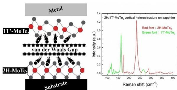
**Low-resistivity Ohmic contacts of Ti/Al on few-layered 1T'-MoTe<sub>2</sub>/2H-MoTe<sub>2</sub> heterojunctions grown by chemical vapor deposition**
