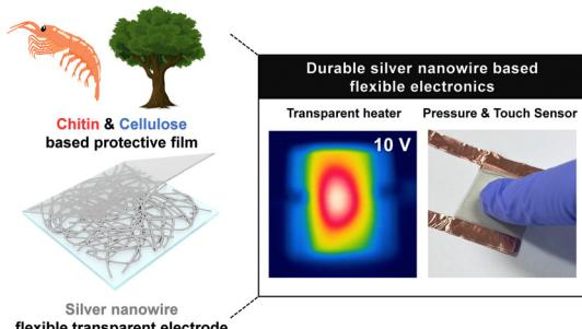
**Durable silver nanowire transparent electrodes enabled by biorenewable nanocoating using chitin and cellulose nanofibers for flexible electronics**
