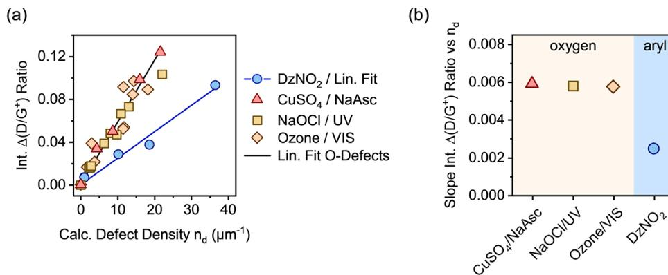
Fig. 3 (a) Integrated Raman  $\Delta(D/G^+)$  ratios versus calculated defect densities ( $n_d$ ) based on PLQY for (6,5) SWCNTs functionalized by different methods creating oxygen or aryl  $sp^3$  defects. Linear fits for oxygen defects, combined ( $R^2 = 0.97$ ) and aryl  $sp^3$  defects ( $R^2 = 0.98$ ). (b) Extracted slopes of the integrated  $\Delta(D/G^+)$  ratio versus calculated defect density for each functionalization method.
