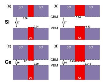
**Fig. 6** Band alignments of (a) bulk 3C-Si and 2L-Si, (b) bulk 3C-Si and 5L-Si, (c) bulk 3C-Ge and 2L-Ge, and (d) bulk 3C-Ge and 5L-Ge.
