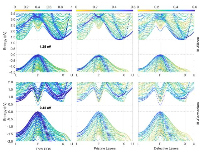
**Fig. 3** 3L-Si and -Ge band structures (top and bottom panels, respectively) unfolded into the primitive cubic cell (colour scale). Energies are plotted relative to the top of the VB. The middle and right panels highlight the different contributions to the band states of the pristine-like and defective atoms (red and plum atoms, respectively, as shown in Fig. 1).
