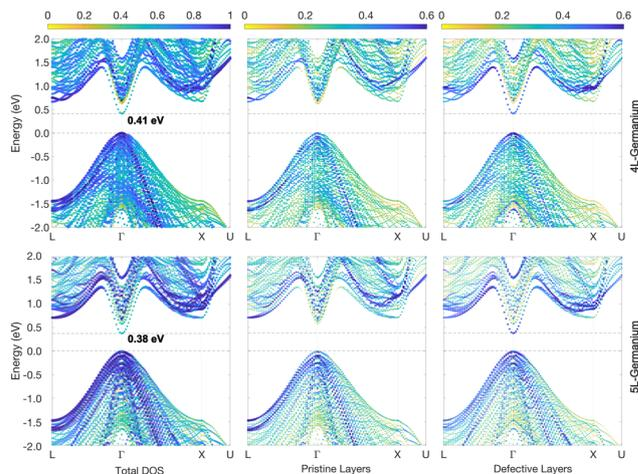
**Fig. 4** 4L-Ge and 5L-Ge band structures (top and bottom panels, respectively) unfolded into the primitive cubic cell (colour scale). Energies are plotted relative to the top of the VB. The middle and right panels highlight the different contributions to the band states of the pristine-like and defective atoms (red and plum atoms, respectively, as shown in Fig. 1).
