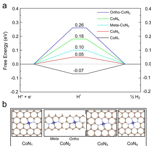
Fig. 5 DFT calculations of hydrogen adsorption. (a) Calculated HER free-energy diagram over different configurations of Co-N<sub>x</sub>-NAC. The H binding energy is labeled on top of each configuration. (b) Atomic structures of H adsorbed on Co-N<sub>x</sub>-NAC.
