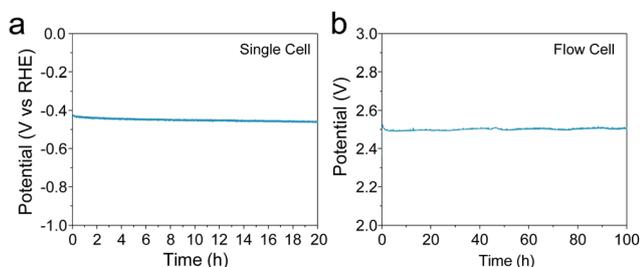
Fig. 4 Stability test of Co-100-NAC-800. (a) Chronopotentiometry (CP) plot showing the stability test at 50 mA cm<sup>-2</sup>; (b) 100-h water-splitting test at 150 mA cm<sup>-2</sup> current density in flow cell with Co-100-NAC-800 as the cathode catalyst and Pt on carbon as the anode catalyst.
