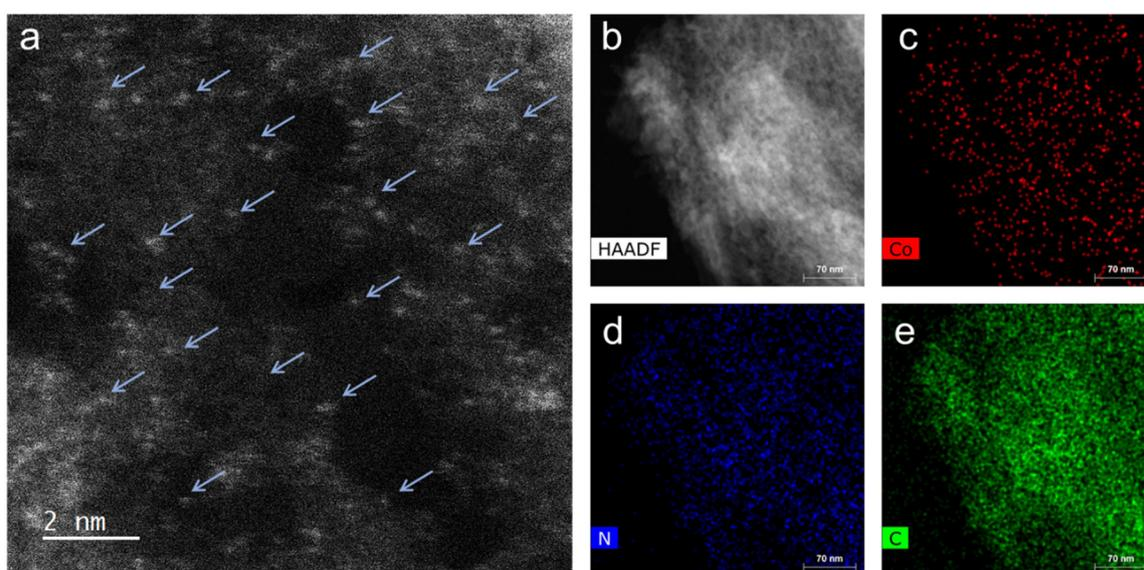
**Fig. 2** Electron-microscopy characterization of Co-100-NAC-800. (a) HR-STEM image of Co-NAC, the arrows indicate the single-atom Co on the NAC support. (b)–(e) EDS elemental mapping images of Co-NAC: (b) HAADF-STEM image; (c) Co mapping; (d) C mapping; (e) N mapping.
