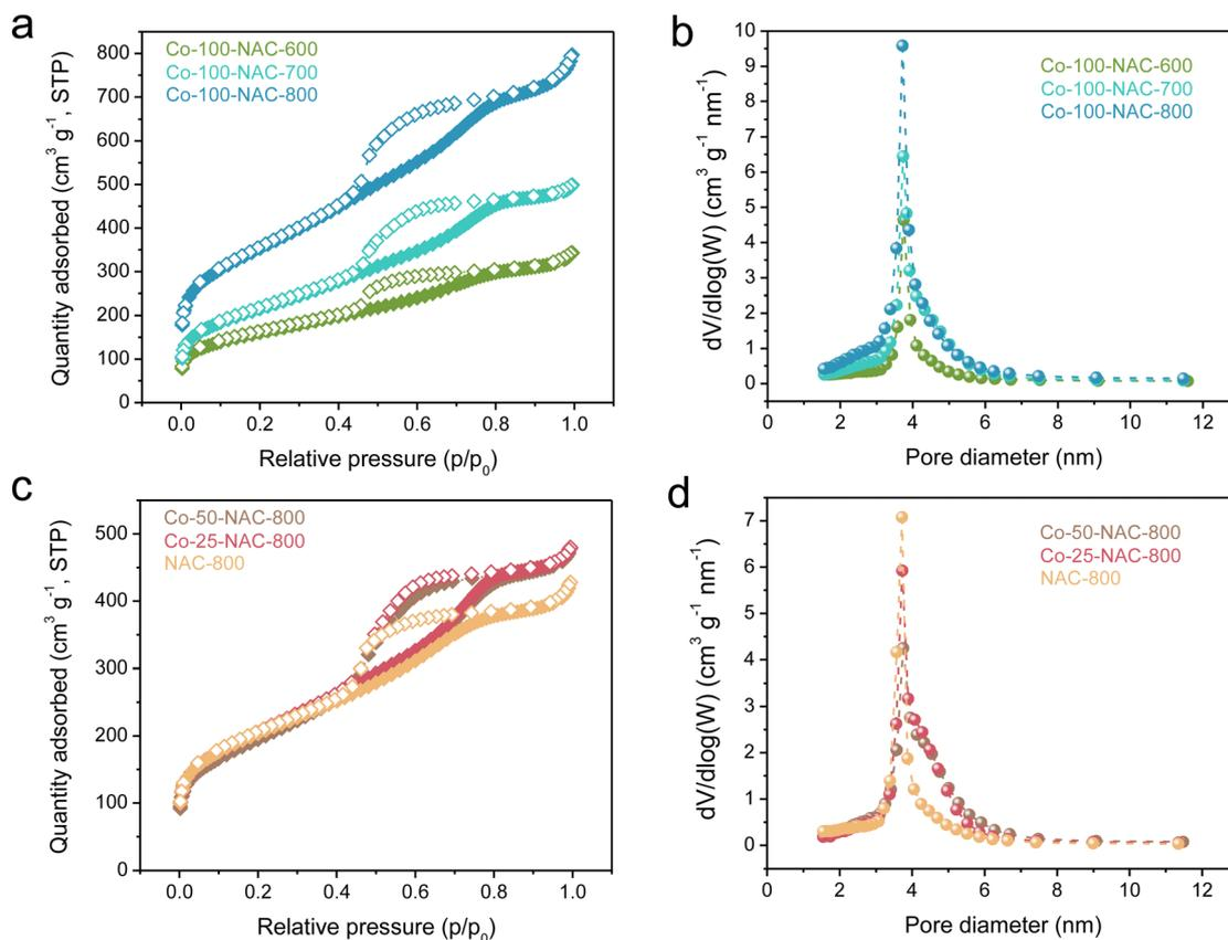
**Fig. 1**  $N_2$ -sorption isotherm (a) and (c) and pore-size distribution (b) and (d) of Co-NAC catalysts carbonized at 600, 700, and 800 °C with different metal loadings. The samples are named as "Co- $x$ -NAC- $y$ ", which are prepared with  $x$  mg of added Co(acac)<sub>2</sub> and under a carbonization temperature of  $y$  °C. The actual Co loadings are summarized in Table S1 (ESI†). NAC-800 is a sample prepared using the same method but without addition of a Co precursor.
