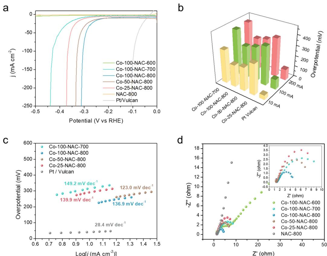
Fig. 3 HER evaluation on Co-NAC. (a) LSV; (b) overpotential at 10, 100, and 200 mA cm<sup>-2</sup>; (c) Tafel plots; (d) Nyquist plots at -0.3 V; insert: zoom-in Nyquist plot. Co-100-NAC-600 overlaps with NAC-800 in (a).
