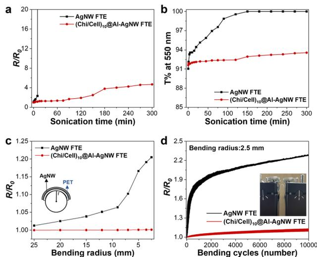
Fig. 5 (a) Relative variation in the electrical resistance and (b) transmittance at 550 nm of AgNW and (Chi/Cell)<sub>10</sub>@Al-AgNW FTEs as a function of sonication time. Relative variation in the electrical resistance of AgNW and (Chi/Cell)<sub>10</sub>@Al-AgNW FTEs as a function of (c) the bending radius and (d) bending cycles at a fixed bending radius of 2.5 mm.
