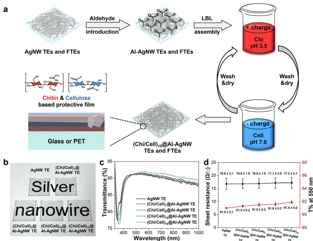
Fig. 1 (a) Schematic diagram for the fabrication of (Chi/Cell)<sub>n</sub>@Al-AgNW TEs and FTEs. (b) Optical images, (c) transmittance spectra, and (d) sheet resistance and transmittance at 550 nm of AgNW, (Chi/Cell)<sub>1</sub>, (Chi/Cell)<sub>5</sub>, (Chi/Cell)<sub>10</sub>, and (Chi/Cell)<sub>15</sub> @Al-AgNW TEs.
