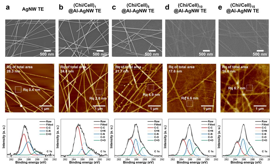
Fig. 2 SEM images, AFM images, *R*<sub>q</sub> of total and squared areas, and C 1s XPS spectra of (a) AgNW, (b) (Chi/Cell)<sub>1</sub>, (c) (Chi/Cell)<sub>5</sub>, (d) (Chi/Cell)<sub>10</sub>, and (e) (Chi/Cell)<sub>15</sub>@Al-AgNW TEs.
